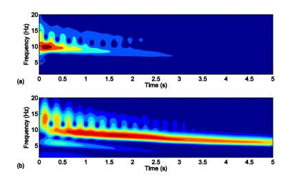
Figure 3.14 Wavelet transform spectra for experimental results with X = 1.42 mm: (a)  $x_p$  and (b)  $x_a$
