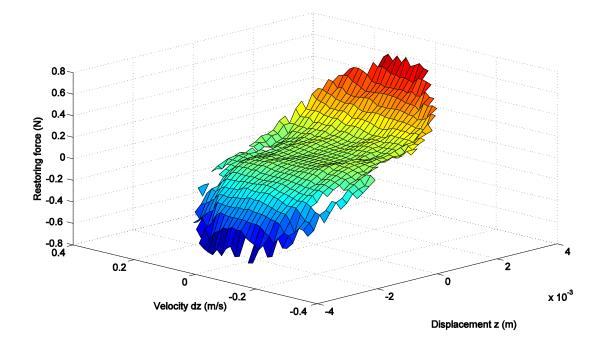
Figure 2.4 Restoring force  $F(z, \dot{z})$  vs. relative displacement z and relative velocity  $\dot{z}$
