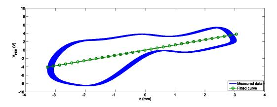
Figure 2.7 Piezoelectric energy harvester voltage vs. relative displacement  $z = x_a - x_p$
