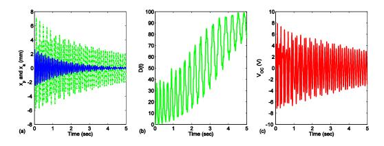
Figure 3.5 Simulation results with X = 2.65 mm: (a) displacements (Solid line: primary system; Dotted line: NES), (b) the percentage of instantaneous energy in NES, and (c) open circuit voltage of PEH.
