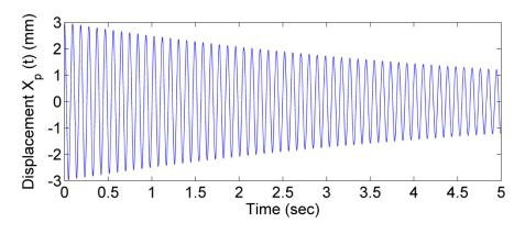
Figure 1.2 Transient response of the primary system:  $x_p(0) = 0.003 m$  and  $\dot{x}_p(0) = 0 m/s$ ,  $m_p = 0.839$  kg,  $k_p = 3799.3$  N/m, and  $c_p = 1.129$  Ns/m
