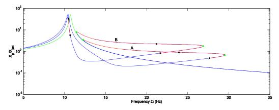
Figure 4.5 Comparison of FRPs for two excitation levels at  $R = 1000 \Omega$ . Curve A obtained with  $A_y = 1.8 \text{ m/s}^2$ ; curve B obtained with  $A_y = 0.6 \text{ m/s}^2$ . Green line represents the FRP of the primary system with NES detached.
