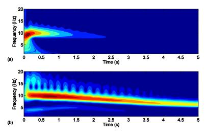
Figure 3.18 Wavelet transform spectra for experimental results with X = 4.45 mm: (a)  $x_p$  and (b)  $x_a$
