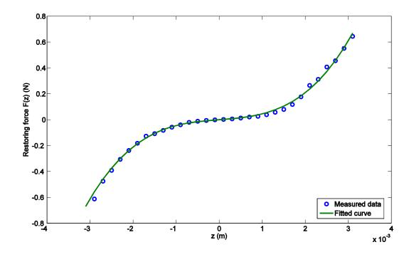
Figure 2.5 Restoring force F(z, 0) vs. displacement z (circle: measured data; line: fitted curved)
