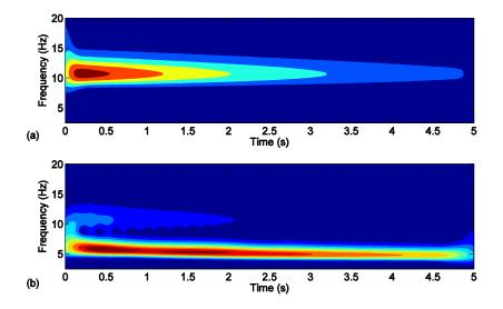
Figure 3.2 Wavelet transform spectra for simulation results with X = 0.52 mm: (a)  $x_p$  and (b)  $x_a$
