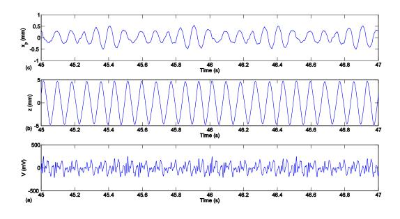
Figure 4.15 Experiment results of displacement response at acceleration  $A_y = 0.6 \text{ m/s}^2$  and  $R = 2000 \Omega$  and excitation frequency  $\Omega = 12 \text{ Hz}$ .
