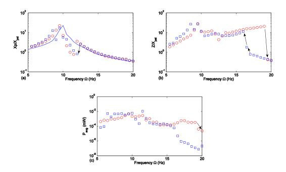
Figure 4.17 Test results with  $A_y = 1.8 \text{ m/s}^2$  and  $R = 1000 \Omega$ . (a)  $X_p/X_{pst}$ , blue line indicates experiment results with NES removed; (b)  $Z/X_{pst}$ ; (c) the average harvested power. (Red circle: forward frequency sweeping; Blue square: backward frequency sweeping.)
