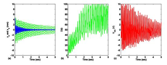
Figure 3.17 Experimental results with X = 4.45 mm: (a) displacements (Solid line: primary system; Dotted line: NES), (b) the percentage of instantaneous energy in NES, and (c) open circuit voltage of PEH.
