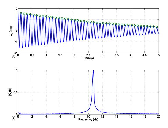
Figure 2.3 Experimental result of primary system: (a) Primary system free response with curve fitted damping curve; (b) FFT plot of free response  $f_p = 10.71$  Hz
