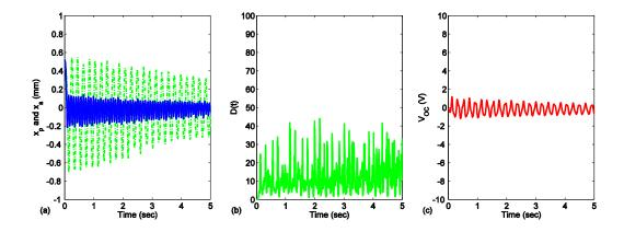
Figure 3.11 Experimental results with X = 0.52 mm: (a) displacements (Solid line: primary system; Dotted line: NES), (b) the percentage of instantaneous energy in NES, and (c) open circuit voltage of PEH.
