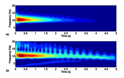
Figure 3.8 Wavelet transform spectra for simulation results with X = 4.45 mm: (a)  $x_p$  and (b)  $x_a$
