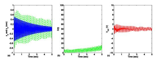
Figure 3.1 Simulation results with X = 0.52 mm: (a) displacements (Solid line: primary; Dotted line: NES), (b) the the percentage of instantaneous energy in NES, and (c) open circuit voltage of PEH
