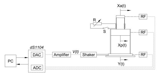
Figure 2.2 Schematic of testing system
