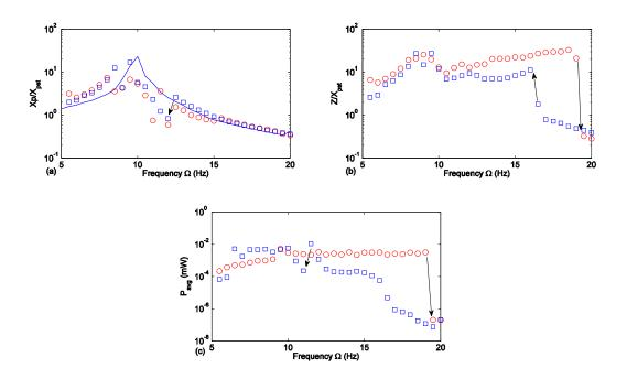
Figure 4.14 Test results with  $A_y = 0.6 \text{ m/s}^2$  and  $R = 2000 \Omega$ . (a)  $X_p/X_{pst}$ , blue line indicates experiment results with NES removed; (b)  $Z/X_{pst}$ ; (c) the average harvested power. (Red circle: forward frequency sweeping; Blue square: backward frequency sweeping.)
