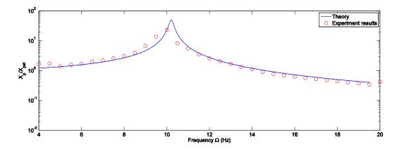
Figure 4.12 Comparison of the analytic T.R. and experimental T.R. of the primary system with  $A_y = 0.6 \text{ m/s}^2$ .
