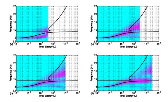
Figure 3.26 Frequency energy plots and wavelet transform of relative displacement  $x_a - x_p$  from the simulation results for  $f_p = 9$  Hz: (a) low initial energy  $X = 0.52 \times 10^{-3}$  (m); (b) medium initial energy  $X = 1.42 \times 10^{-3}$  (m); (c) medium-high initial energy  $X = 2.65 \times 10^{-3}$  (m) and (d) high initial energy  $X = 4.45 \times 10^{-3}$  (m).
