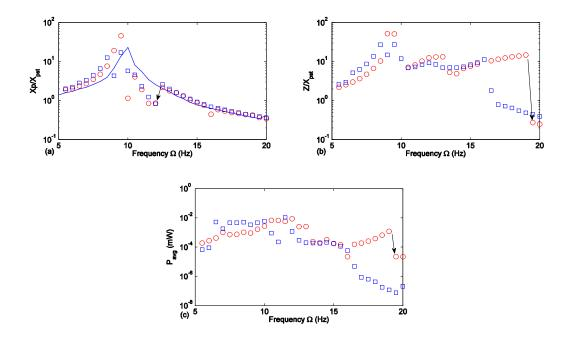
Figure 4.13 Test results with  $A_y = 0.6 \text{ m/s}^2$  and  $R = 1000 \Omega$ . (a)  $X_p/X_{pst}$ , blue line indicates the experiment results with the NES removed; (b)  $Z/X_{pst}$ ; (c) the average harvested power. (Red circle: forward frequency sweeping; Blue square: backward frequency sweeping.)
