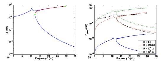
Figure 4.10 Relative displacement and peak power with  $A_y = 1.8 \text{ m/s}^2$ . (a) FRP for relative displacement and (b) peak power as a function of frequency at  $R = 0, 1000, 10^5, 10^7 \Omega$ .
