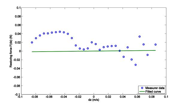
Figure 2.6 Restoring force  $F(0, \dot{z})$  vs. velocity  $\dot{z}$  (circle: measured data; line: fitted curved)
