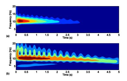
Figure 3.6 Wavelet transform spectra for simulation results with X = 2.65 mm: (a)  $x_p$  and (b)  $x_a$
