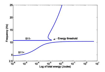
Figure 3.20 Frequency energy plot: backbone curves S11±
