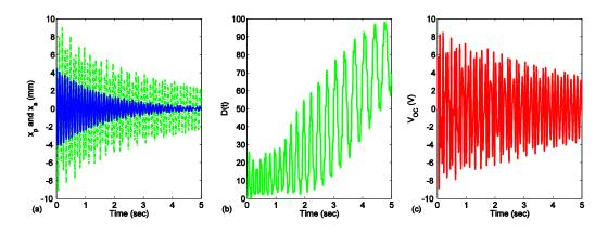
Figure 3.7 Simulation results with X = 4.45 mm: (a) displacements (Solid line: primary system; Dotted line: NES), (b) the percentage of instantaneous energy in NES, and (c) open circuit voltage of PEH.
