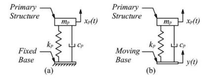
Figure 1.1 Schematic of two vibration problems: (a) transient response due to initial disturbance; (b) harmonic base excitation.
