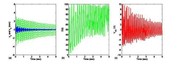
Figure 3.13 Experimental results with X = 1.42 mm: (a) displacements (Solid line: primary system; Dotted line: NES), (b) the percentage of instantaneous energy in NES, and (c) open circuit voltage of PEH.
