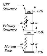
Figure 1.4 Schematic of a NES attached to a primary system subjected to base excitation.
