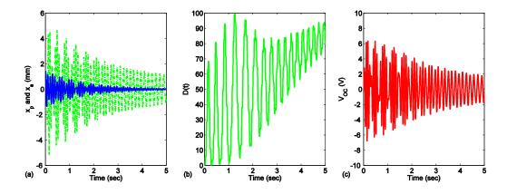
Figure 3.3 Simulation results with X = 1.42 mm: (a) displacements (Solid line: primary system; Dotted line: NES), (b) the percentage of instantaneous energy in NES, and (c) open circuit voltage of PEH.
