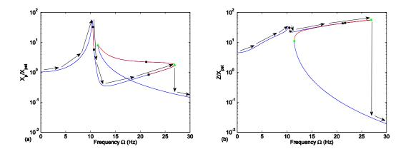
Figure 4.3 FRPs obtained by forward frequency sweeping with  $A_y = 0.6 \text{ m/s}^2$ : arrows indicate the response path. (a)  $X_p/X_{pst}$ , (b)  $Z/X_{pst}$
