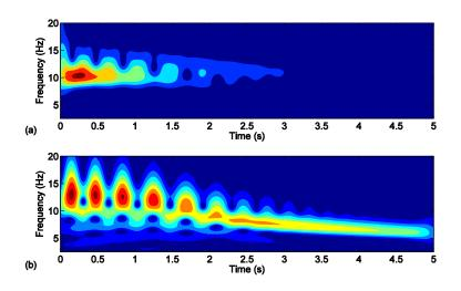
Figure 3.4 Wavelet transform spectra for simulation results with X = 1.42 mm: (a)  $x_p$  and (b)  $x_a$
