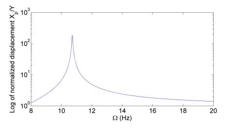
Figure 1.3 Displacement ratio of system:  $f_n = 10.71$  Hz
