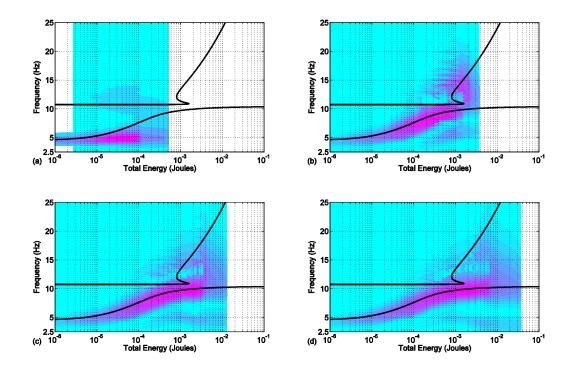
Figure 3.22 Frequency energy plots and wavelet transforms of relative displacement  $x_a - x_p$  from the experimental results for  $f_p = 10.71$  Hz: (a) low initial energy  $X = 0.52 \times 10^{-3}$  (m); (b) medium initial energy  $X = 1.42 \times 10^{-3}$  (m); (c) medium-high initial energy  $X = 2.65 \times 10^{-3}$  (m) and; (d) high initial energy  $X = 4.45 \times 10^{-3}$  (m).
