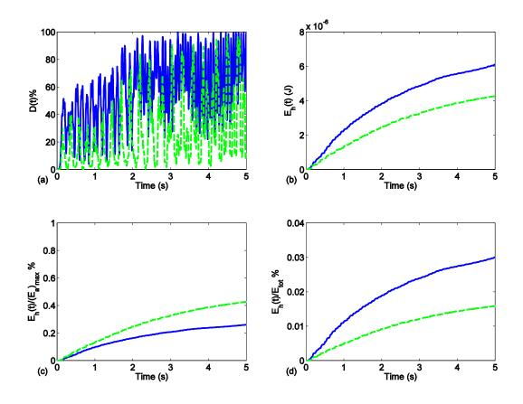
Figure 3.24 Experimental results of non-dimensional system: (a) the percentage of instantaneous energy in NES, (b) accumulated energy in NES, (c) ratio of accumulated energy in NES to maximum of kinetic energy in NES, and (d) ratio of accumulated energy in NES to total system energy, (solid blue line:  $\eta = 0.3$  or  $f_p = 15$  Hz, dash green line:  $\eta = 0.5$  or  $f_p = 9$  Hz).
