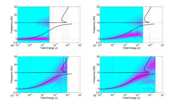
Figure 3.28 Frequency energy plots and wavelet transforms of relative displacement  $x_a - x_p$  from the simulation results for  $f_p = 15$  Hz: (a) low initial energy  $X = 0.312 \times 10^{-3}$  (m); (b) medium initial energy  $X = 0.852 \times 10^{-3}$  (m); (c) medium-high initial energy  $X = 1.59 \times 10^{-3}$  (m) and (d) high initial energy  $X = 2.67 \times 10^{-3}$  (m).
