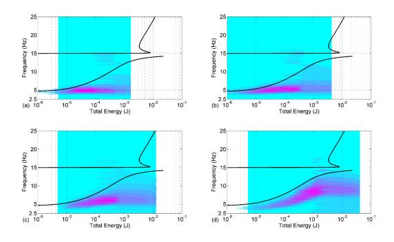
Figure 3.29 Frequency energy plots and wavelet transforms of relative displacement  $x_a - x_p$  from the experimental results for  $f_p = 15$  Hz: (a) low initial energy  $X = 0.312 \times 10^{-3}$  (m); (b) medium initial energy  $X = 0.852 \times 10^{-3}$  (m); (c) medium-high initial energy  $X = 1.59 \times 10^{-3}$  (m) and (d) high initial energy  $X = 2.67 \times 10^{-3}$  (m).
