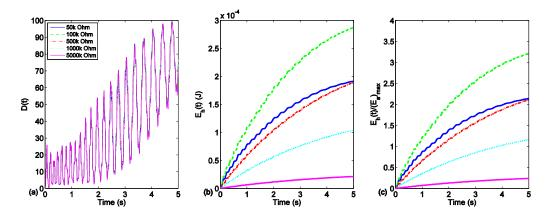
Figure 3.9 Simulation results with X = 4.45 mm: (a) the percentage of instantaneous energy in NES, (b) accumulated energy in NES, and (c) ratio of accumulated energy in NES to maximum of kinetic energy of NES.
