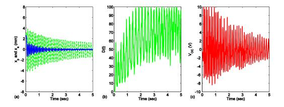
Figure 3.15 Experimental results with X = 2.65 mm: (a) displacements (Solid line: primary system; Dotted line: NES), (b) the percentage of instantaneous energy in NES, and (c) open circuit voltage of PEH.
