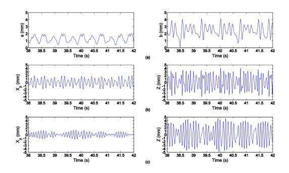
Figure 4.2 Time response of strongly modulated response with  $A_y = 0.6 \text{ m/s}^2$ ,  $R = 1000 \Omega$ , and  $\Omega = 10.58$  Hz: (a) amplitudes by solving Equations (4.32) to (4.35) with Matcont; (b) reconstituted responses defined by Equations (4.36) and (4.37); (c) responses by numerically integrating Equations (4.1) to (4.3).
