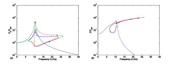
Figure 4.8 Closed island and FRP at  $A_y = 0.3 \text{ m/s}^2$ . (a)  $X_p/X_{pst}$ , (b)  $Z/X_{pst}$ . Green line represents the primary system with NES detached.
