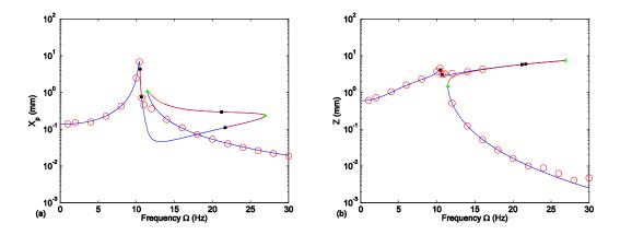
Figure 4.1 FRP for  $A_y = 0.6 \text{ m/s}^2$  and  $R = 1000 \Omega$ : (a) primary displacement  $X_p$  and (b) relative displacement Z. Blue line indicates stable periodic orbits. Red lines are unstable indicating non-periodic orbits. Black squares are Hopf bifurcation points and green triangles are Limit points. Red circles are from numerical integration of Equations (4.1) to (4.3)
