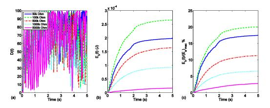
Figure 3.19 Experimental results with X = 4.45 mm: (a) the percentage of instantaneous energy in NES, (b) accumulated energy in NES, and (c) ratio of accumulated energy in NES to maximum of kinetic energy of NES.
