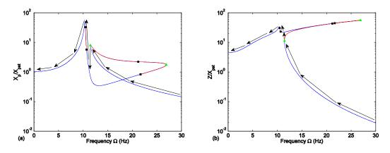
Figure 4.4 FRPs obtained by backward frequency sweeping with  $A_y = 0.6 \text{ m/s}^2$ : arrows indicate the response path. (a)  $X_p/X_{pst}$ , (b)  $Z/X_{pst}$
