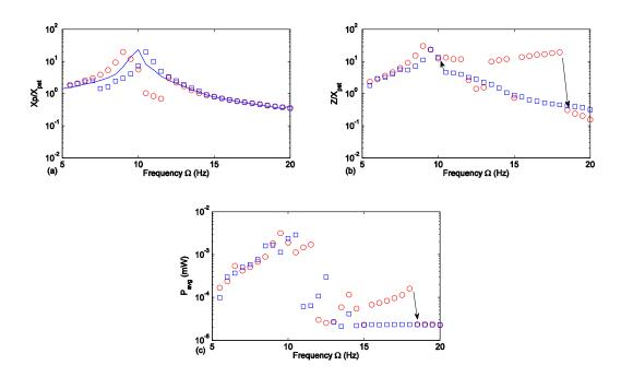
Figure 4.16 Test results with  $A_y = 1.2 \text{ m/s}^2$  and  $R = 1000 \Omega$ . (a)  $X_p/X_{pst}$ , blue line indicates experiment results with NES removed; (b)  $Z/X_{pst}$ ; (c) the average harvested power. (Red circle: forward frequency sweeping; Blue square: backward frequency sweeping.)
