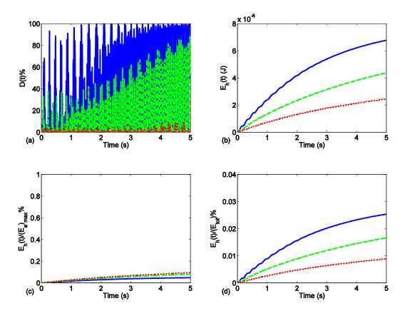
Figure 3.23 Simulation results of non-dimensional system: (a) the percentage of instantaneous energy in NES, (b) accumulated energy in NES, (c) ratio of accumulated energy in NES to maximum of kinetic energy in NES, and (d) ratio of accumulated energy in NES to total system energy, (solid blue line:  $\eta = 0.3 \text{ or } f_p = 15 \text{ Hz}$ , dash green line:  $\eta = 0.5 \text{ or } f_p = 9 \text{ Hz}$ , and red dotted line:  $\eta = 1 \text{ or } f_p = 4.5 \text{ Hz}$ ).
