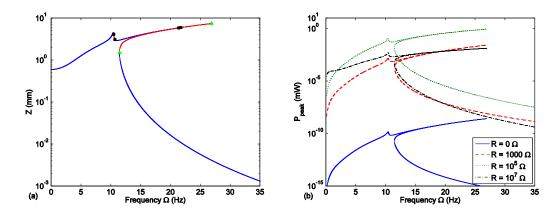
Figure 4.9 Relative displacement and peak power at acceleration  $A_y = 0.6 \text{ m/s}^2$ . (a) FRP for relative displacement and (b) peak power as a function of frequency at  $R = 0, 1000, 10^5, 10^7 \Omega$ .
