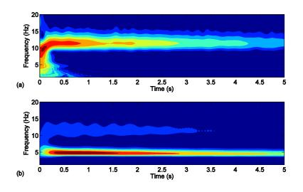
Figure 3.12 Wavelet transform spectra for experimental results with X = 0.52 mm: (a)  $x_p$  and (b)  $x_a$
