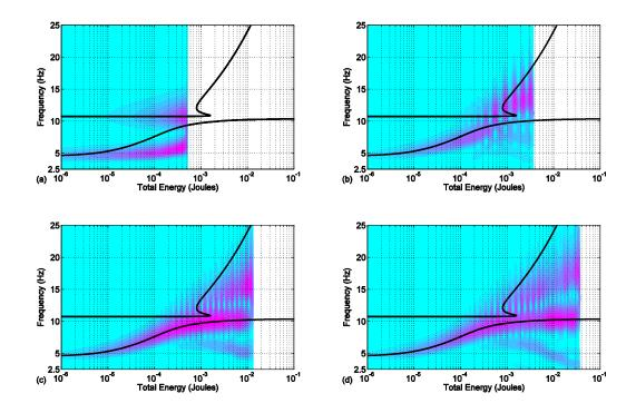
Figure 3.21 Frequency energy plots and wavelet transforms of relative displacement  $x_a - x_p$  from the simulation results for  $f_p = 10.71$  Hz: (a) low initial energy  $X = 0.52 \times 10^{-3}$  (m); (b) medium initial energy  $X = 1.42 \times 10^{-3}$  (m); (c) medium-high initial energy  $X = 2.65 \times 10^{-3}$  (m) and; (d) high initial energy  $X = 4.45 \times 10^{-3}$  (m).
