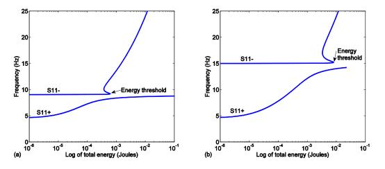
Figure 3.25 Frequency energy plot: backbone curves  $S11\pm$  for (a)  $f_p = 9$  Hz, (b)  $f_p = 15$  Hz
