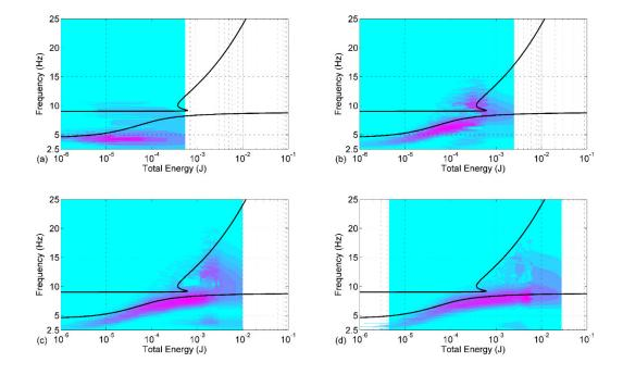
Figure 3.27 Frequency energy plots and wavelet transforms of relative displacement  $x_a - x_p$  from the experimental results for  $f_p = 9$  Hz: (a) low initial energy  $X = 0.52 \times 10^{-3}$  (m); (b) medium initial energy  $X = 1.42 \times 10^{-3}$  (m); (c) medium-high initial energy  $X = 2.65 \times 10^{-3}$  (m) and (d) high initial energy  $X = 4.45 \times 10^{-3}$  (m).
