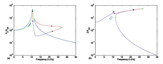
Figure 4.7 Closed island and FRP at  $A_y = 0.6 \text{ m/s}^2$ . (a)  $X_p/X_{pst}$ . (b)  $Z/X_{pst}$ . Green line represents the primary system with NES detached.
