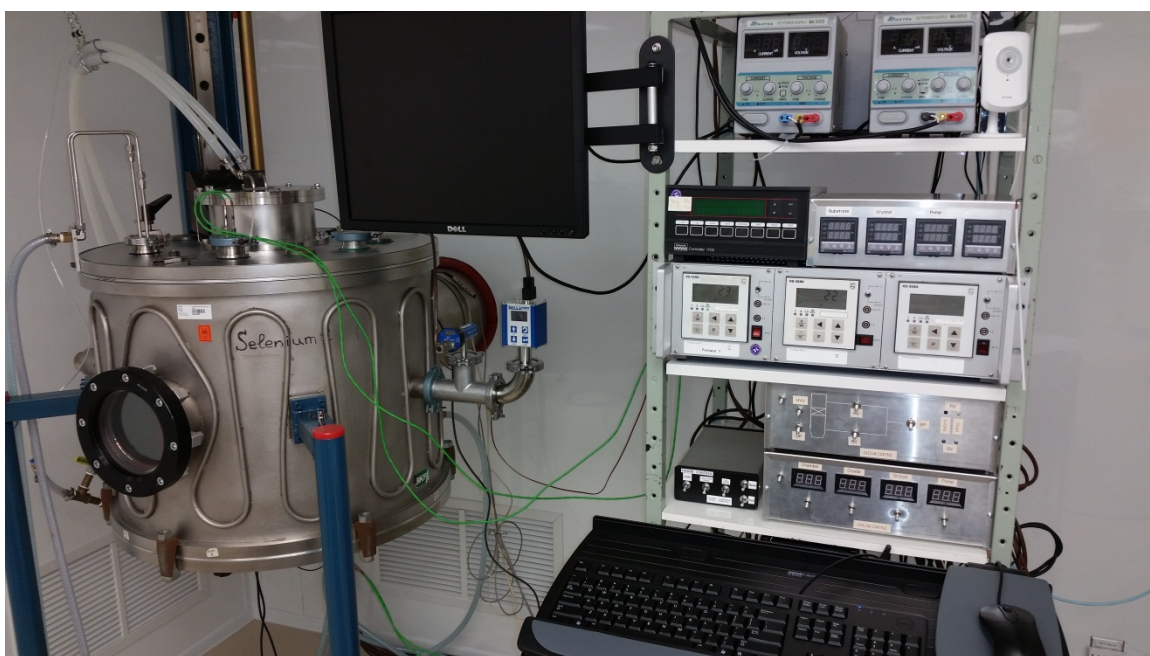
Figure 51. Vacuum deposition system utilized for a-Se deposition in Thunder Bay Regional Research Institute clean rooms facilities.
