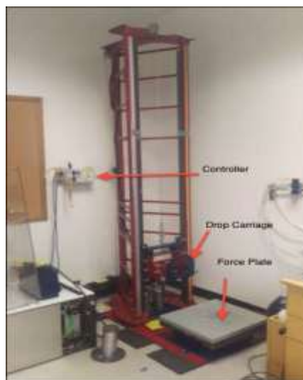
Figure 7. Lakehead University drop system. The controller can be seen to the left of the system. The forward/reverse switch to control raising and lowering is attached by cable to the controller. The neck and headform are mounted, along with the circular steel plate, to the circular blue plate seen above.
