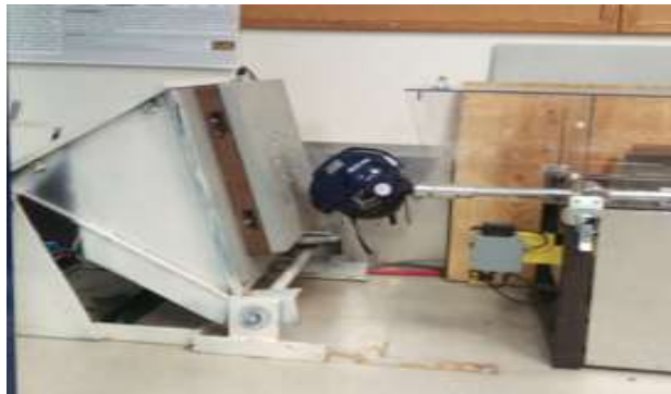
Figure 10. Repetitive impactor used to measure helmet deterioration. The helmet is mounted to a headform and piston that can repetitively impact the helmet against the previously described AMTI forceplate.
