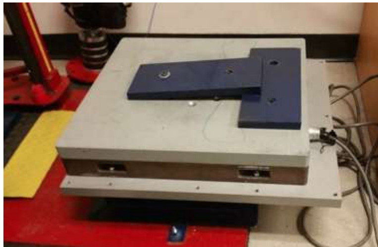
Figure 8. AMTI force platform. This figure shows the force platform with a wedge mounted on the surface to achieve an impact angle of 13.5 degrees.
