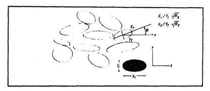
Fig. 4-2 Ellipses from Figure 4-1 deformed by a homogeneous strain  $(R_{+})^{\frac{1}{2}}$ . (From Ramsay, 1967).
