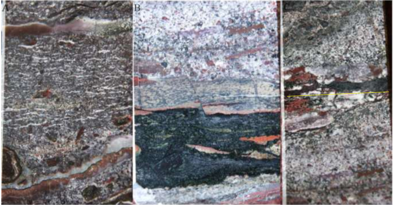
Figure 139: Photographs of the non-oolitic layer present in the oolitic section of the drill core. A) The lower oncolite-poor grainstone layer featuring the horizontal chert filled fractures. B) The magnetite layer at the bottom of the second oncolite-poor sub-stratigraphic unit of the oncolite stratigraphic unit. C) The chert vein between the grainstones of the upper oncolite-poor sub-stratigraphic unit. The PR98-1 drill cores diameter is 4.6cm
