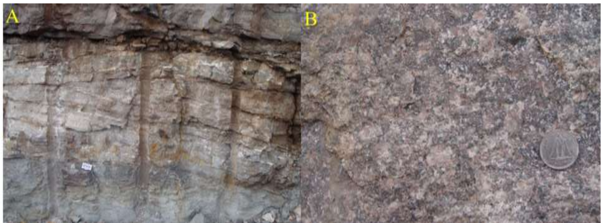
Figure 7: The unaltered layer from the Highway 11/17 outcrop. A) The entire unaltered stratigraphic unit of the 11/7 outcrop grading up into the altered layer. B) Close up of the unaltered granodiorite showing the pink potassium feldspar and waxy plagioclase with minor amounts of quartz and biotite.
