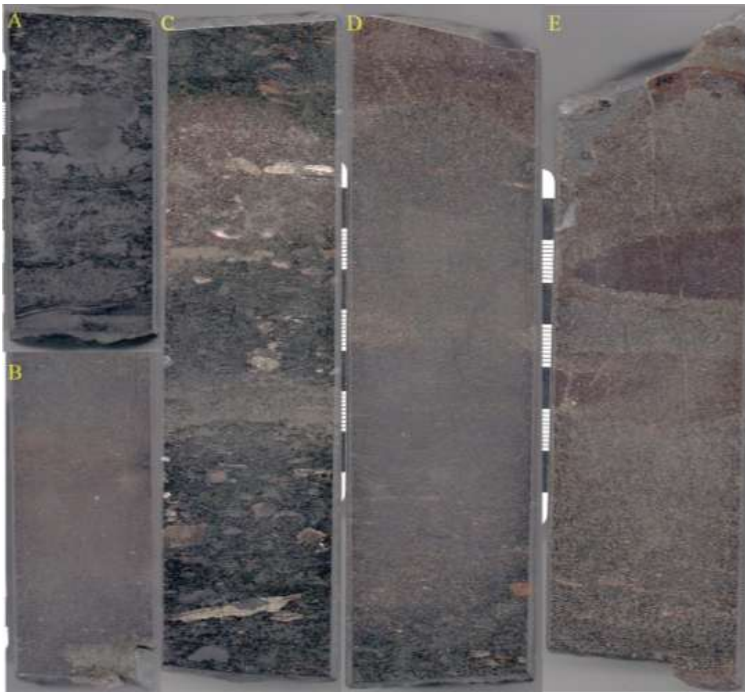
Figure 143: The grainstone section that caps off the PR98-1 sequence. Sample PR98-23 came from this layer. The PR98-1 drill core has a diameter of 4.6 cm
