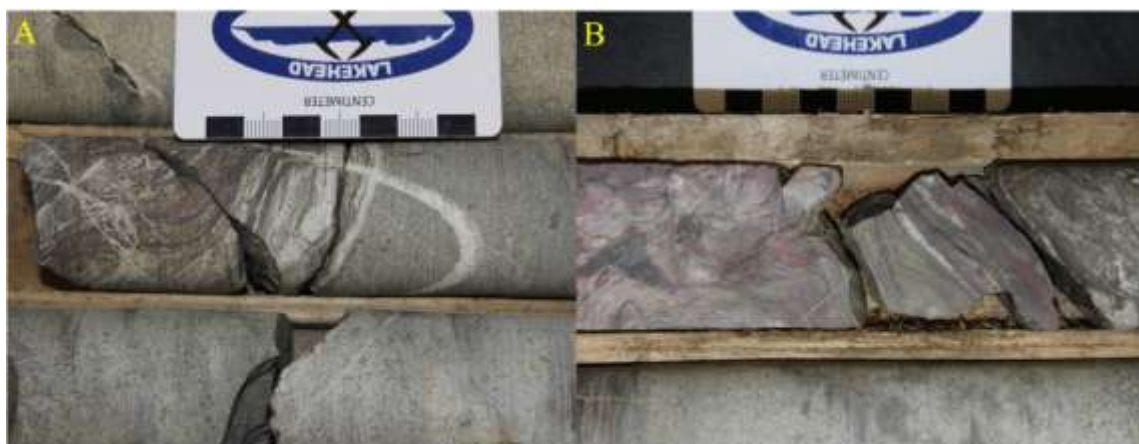
Figure 80: Core photos of the stromatolites from drill hole 87-3. A) The contact between the grainstone and stromatolites. B) The red stromatolites
