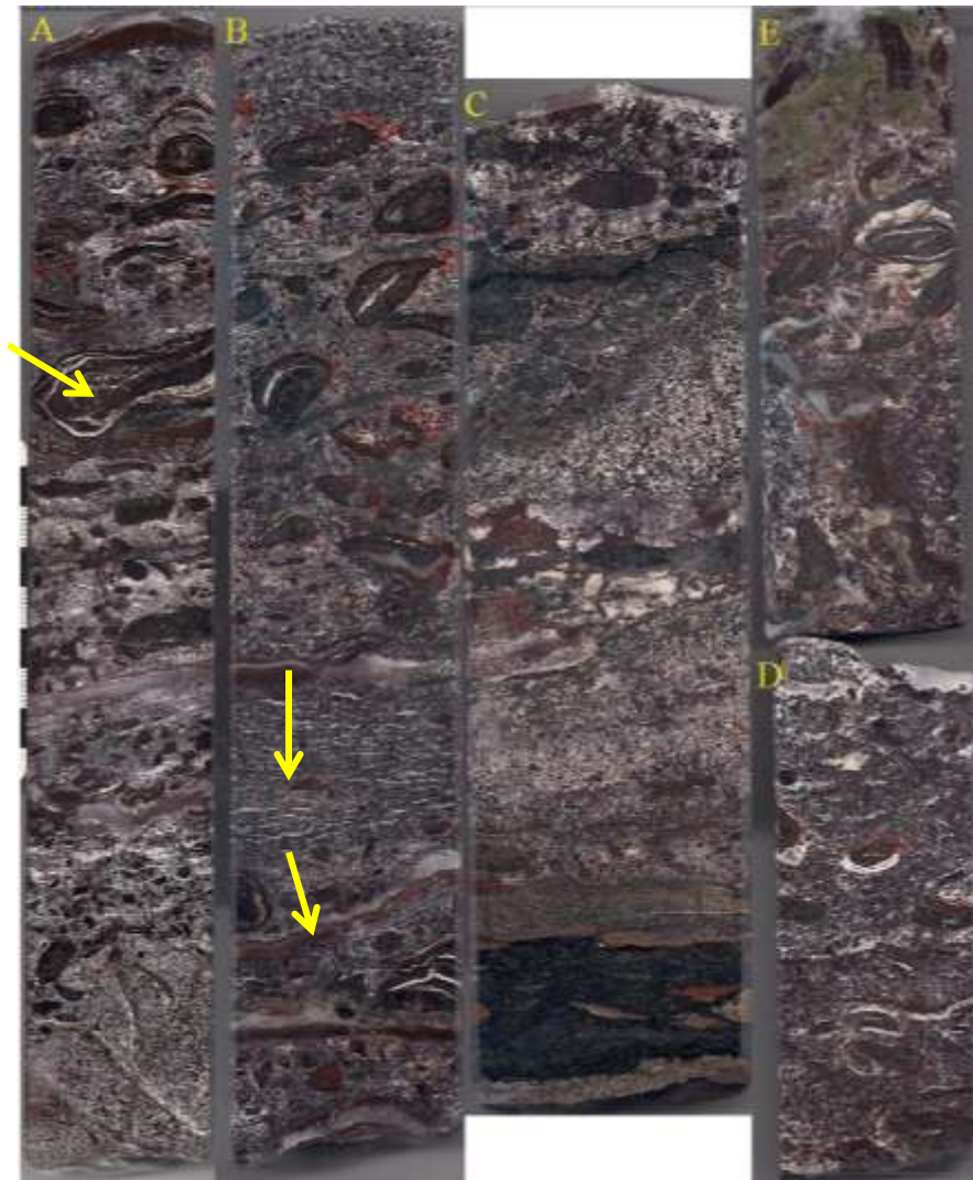
Figure 137: The oncolite stratigraphic unit from the PR98-1 drill hole. A) The bottom of the oncolite stratigraphic unit showing the largest oncolite (yellow) present directly above the brecciated stratigraphic unit. B) The next layer of the oncolite stratigraphic unit, showing the first of the oncolite poor layers (yellow arrows). C) The second and larger non-oncolitic layer. D) The re-emergence of oncolite deposition E) The top of the oncolite layer showing the appearance of the massive green ferroactinolite layer. Samples from here are PR98-6, PR98-7, PR98-10, PR98-11. The drill core has a diameter of 4.6 cm.
