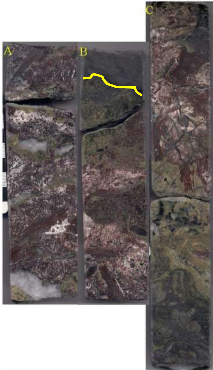
Figure 140: Images of the green brecciated layer from the drill core PR98-1. A) The start of the stratigraphic unit comprised of mostly grainstone with quartz blobs in which the ferroactinolite is present at the bottom of each blob. B) The contact with the fine grained calcite and ferroactinolite. C) Brecciation of the grainstones. Medium to coarse grainstone is fractured by quartz filled veins. Drill core geochemistry samples from here are PR98-12, PR98-13, PR98-14, PR98-15, PR98-16, and PR98-17. PR98-1 drill core has a diameter of 4.6cm.
