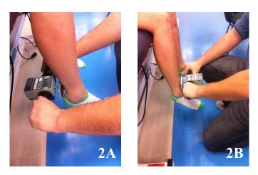
*Figure 2-* (A) This represents the posterior position of the dynamometer over the distal portion of the affected leg. (B) This represents the anterior position of the dynamometer over the distal portion of the affected leg.
