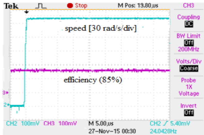
Fig. 5.6: Experimental speed and efficiency responses of the proposed DTFC at rated speed and 50% rated load.
