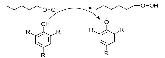
Scheme 1-3: Simple example of stabilization by a chain breaking donor. The radical in the donor is subsequently stabilized through resonance and/or steric hindrance or two donors will stabilize each other. Adapted from reference 53.
