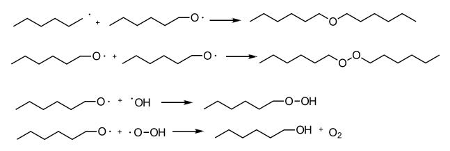
Scheme I-27: Multiple reaction pathways for termination with alkoxy to occur. Although the free radical is terminated, some species may continue to react; adapted from reference 3.
