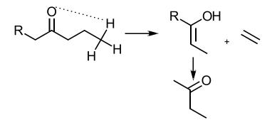
Scheme I-24: Norrish Type II reaction, which occurs as a result of photo-oxidative degradation; adapted from reference 7.
