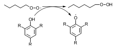
Scheme I-31: Simple example of stabilization by chain breaking donors, the radical in the antioxidant is then stabilized through resonance and/or steric hindrance or two antioxidants will stabilize each other; adapted from reference 9.
