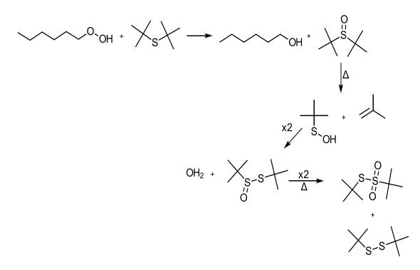
Scheme 1-6: Sulphides inhibit reactions by preventing further reactions. They are not initially stabilizers, but become stabilizers during autoxidation. Adapted from reference 34.
