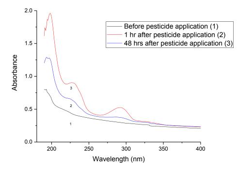
Figure 3-8: UV absorbance of PE film after application of  $0.0066 \pm 0.0005$  g of Pyrinex 480 per m<sup>2</sup> of film.
