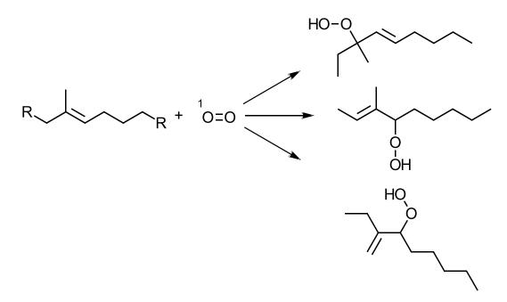
Scheme I-3: Singlet oxygen can occur from energy transfer from photo excited sensitizers; adapted from reference 3.
