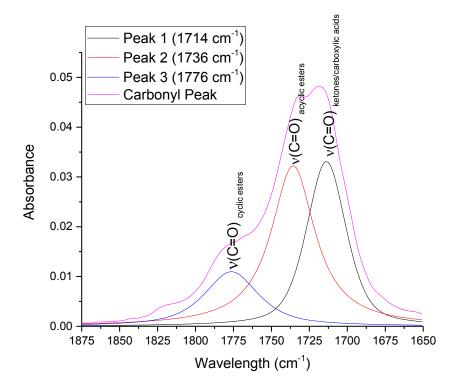
Figure 3-2: A portion of an absorbance spectrum measured for a film (without pesticide application) after 35 hours spent in the SEPAP device. The region between 1650 and 1875 cm<sup>-1</sup> is shown to highlight the multiple peaks in the 1715 cm<sup>-1</sup> region,  $R^2$ =0.999501.
