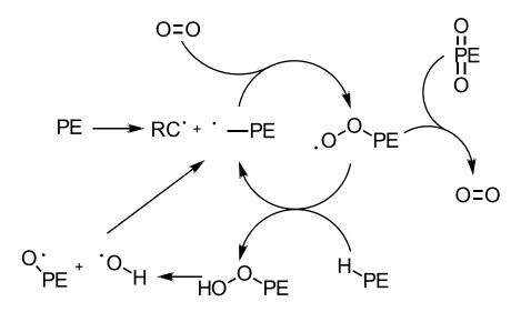
Scheme 1-1: Overall mechanism of PE degradation. Adapted from reference 34.
