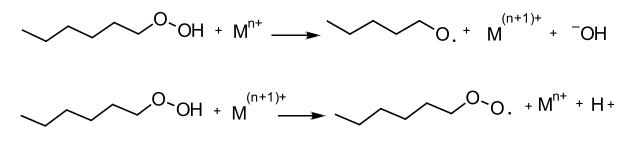
Scheme 1-7: Redox reactions in the PE structure where M represents a transition metal prodegradant. Adapted from reference 9.
