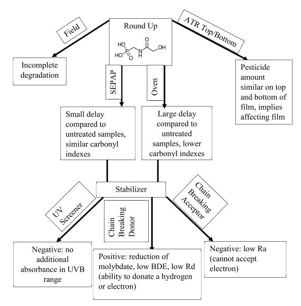
Figure 3-16 : Flow chart demonstrating process of classifying how Round Up may affect degradation.
