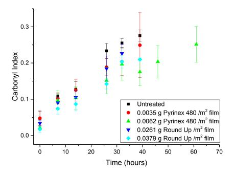
Figure 3-11: The change in carbonyl index over hours of exposure in the SEPAP for samples with and without applied pesticide. The error bars indicate the standard deviation between a minimum of two samples.
