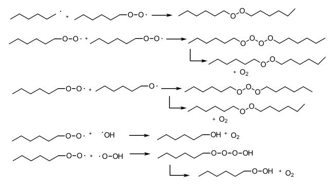
Scheme I-28: Multiple reaction pathways for termination to with peroxyls occur. Although the free radical is terminated; some species may continue to react; adapted from reference 3.
