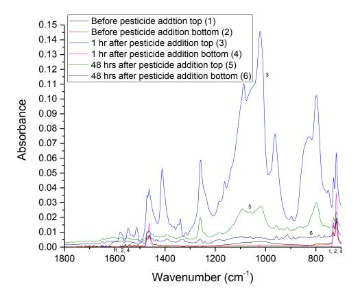
Figure 3-6: ATR spectra of PE film after addition of  $0.0066 \pm 0.0005$  g of Pyrinex 480 per m<sup>2</sup> of film without degradation exposure.
