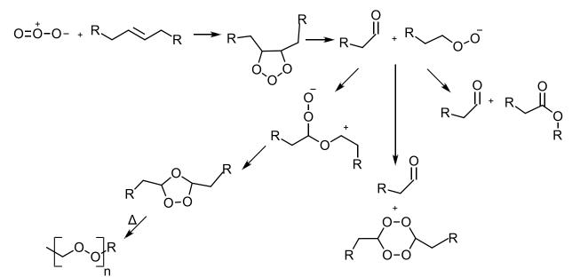
Scheme I-5: The incorporation of oxygen into the film from ozone, a natural result of weathering; adapted from references 1,3.
