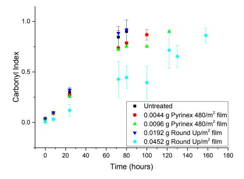
Figure 3-13: The carbonyl index over hours of exposure in the oven at 70 °C for samples with and without applied pesticide. Error bars represent the standard deviation between a minimum of two samples.
