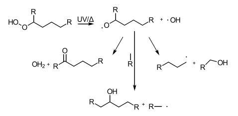
Scheme I-5: The cleavage of the hydroperoxide bond forming new functional groups or scission of the beta bond; adapted from reference 4.
