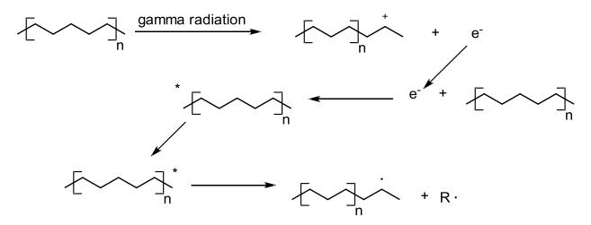
Scheme I-1: High energy breaks carbon- carbon or carbon- hydrogen bonds, rate of degradation depends on oxygen and antioxidants present; adapted from reference 1.
