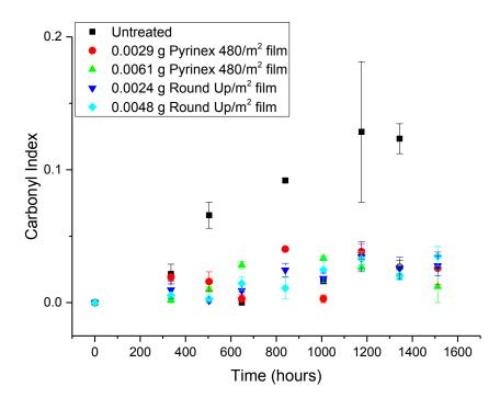
Figure 3-10: The difference in carbonyl index versus exposure time in the field. Error bars represent the standard deviation between two different samples. Each sample was a unique piece of film as samples could not be replaced in the field.
