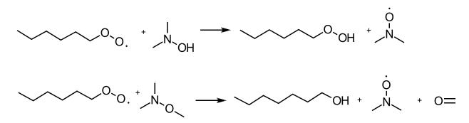
Scheme I-32: Reactions typical of hindered amine stabilizers. The formed amine radical can then take part in secondary antioxidant reactions; adapted from reference 5.
