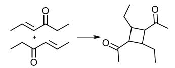
Scheme I-22: Two ketones with unsaturation may result in crosslinking; adapted from reference 3.
