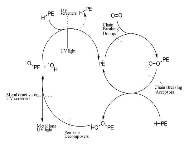
Scheme 1-2: Different degradation mechanisms of PE, indicating by dashed lines where stabilizers can affect degradation. Adapted from reference 34.
