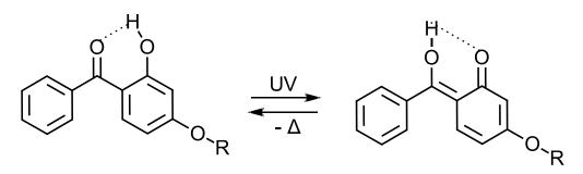
Scheme I-30: The abstraction of hydrogen from the phenol by the ketone with thermal energy loss has been seen to account for the UV screening effect; adapted from reference 1.
