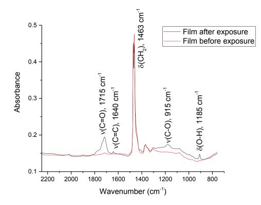
Figure 3-1: IR absorbance in transmission mode of a PE film prior to and after 35 hours in the SEPAP device. The same piece of film was measured.
