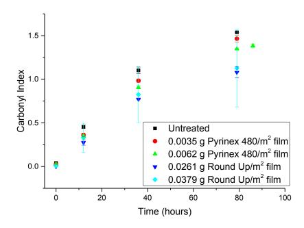
Figure 3-14: The carbonyl index as a function of exposure time in the oven at 80 °C for samples with and without applied pesticide. Error bars represent the standard deviation between a minimum of two samples.
