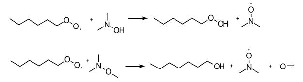
Scheme 1-4: Reactions typical of hindered amine stabilizers. The formed amine radical can then take part in secondary reactions. Adapted from reference 52.
