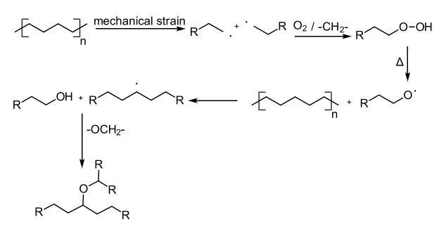
Scheme I-4: Mechanical stress in the polymer induces strain which causes crosslinking and some chain scission; adapted from reference 1.
