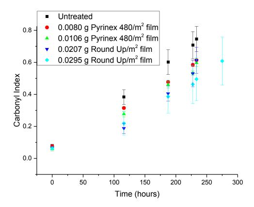
Figure 3-12: The carbonyl index as a function of exposure time in the oven at 60 °C for samples with and without applied pesticide. Error bars represent the standard deviation between a minimum of two samples.
