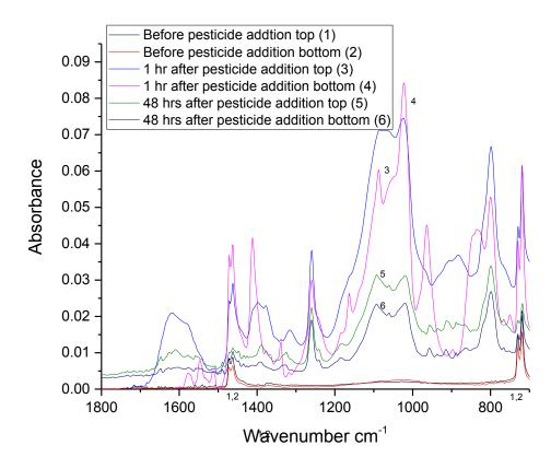
Figure 3-7: ATR spectrum of PE film after addition of  $0.0261 \pm 0.0005$  g of Round Up per m<sup>2</sup> of film without degradation exposure.
