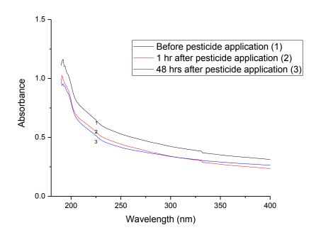
Figure 3-9: UV absorbance of PE film after application of  $0.0261 \pm 0.0005$  g of Round Up per m<sup>2</sup> of film.
