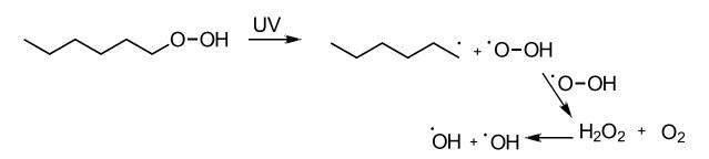
Scheme I-7: Hydroperoxides can be broken into hydroperoxyl radicals. These may react to form hydrogen peroxide which can undergo photolysis to produce hydroxyl radicals; adapted from reference 3.
