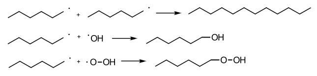
Scheme I-29: Multiple reaction pathways for termination with alkyls to occur. Although the free radical is terminated, some species may continue to react; adapted from reference 3.
