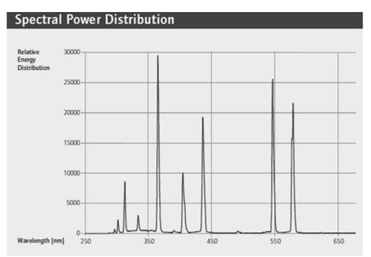
Figure 2-3: The spectral power of the SEPAP 12/24. Peak maximums are found at 290, 313, 365, 405, 436, 547 and 579 nm. Reproduced from reference <sup>31</sup>.
