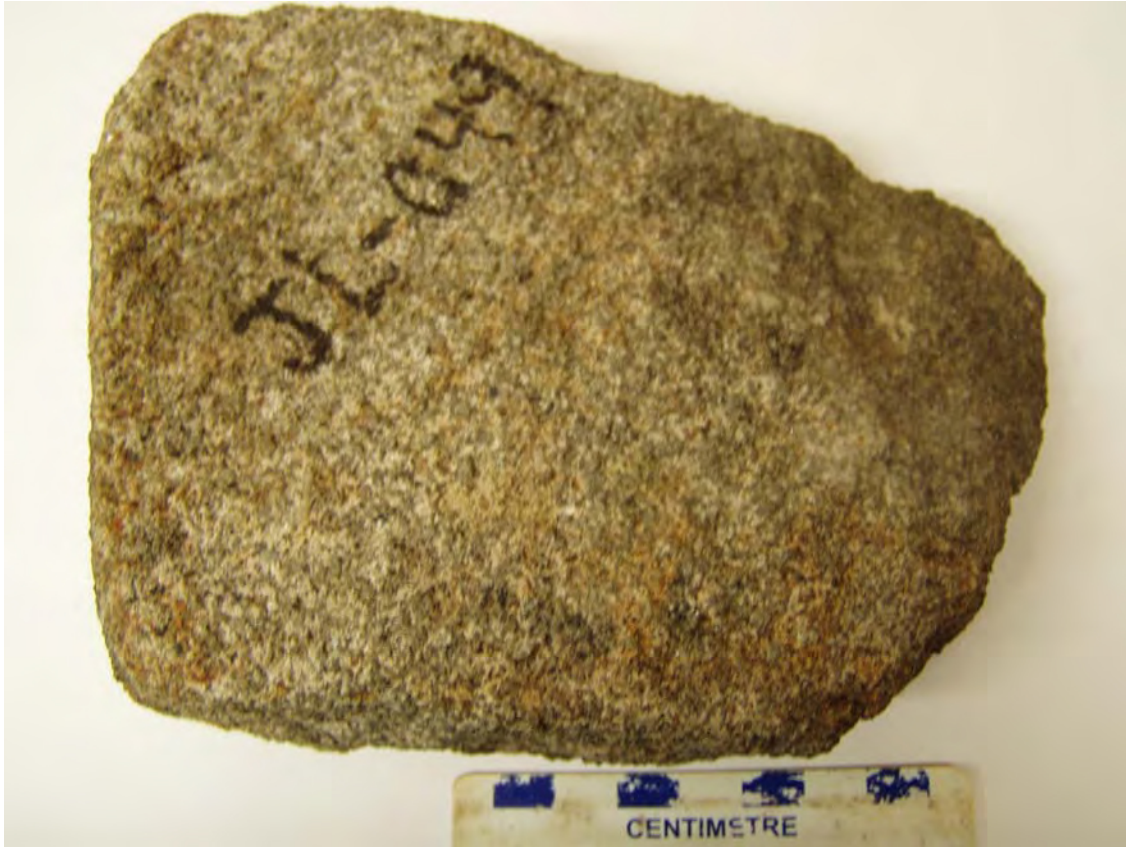
Figure 3.36: In hand sample, Nipigon diabase is massively textured and contains very fine to fine grained ophitic associations of plagioclase and pyroxene. Oxide minerals are fine to medium grained anhedral phases.
