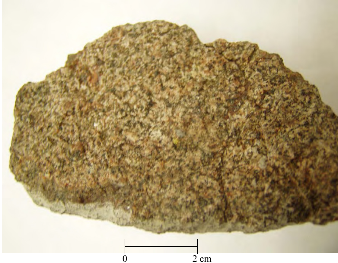
Figure 3.34: In hand sample granophyric gabbro displays a massive coarse grained leucocratic texture. Large, up to 1.5 cm, laths of feldspar to rounded 1 to 2 mm crystals surround elongate up to 2 cm acicular crystals of pyroxene.
