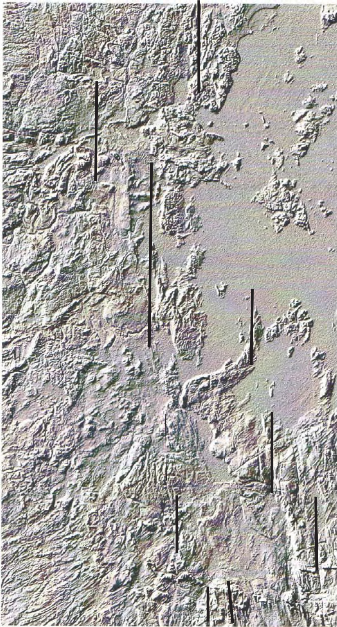
Figure 2.9: A topographic relief map of the West Nipigon Embayment displays many northwest to north-south orientated topographic lineaments indicative of faults and the north to northwest orientated nature of intrusion of diabase dikes and sills. Trends of lineaments are indicated by lines. Modified from OGS (2004).
