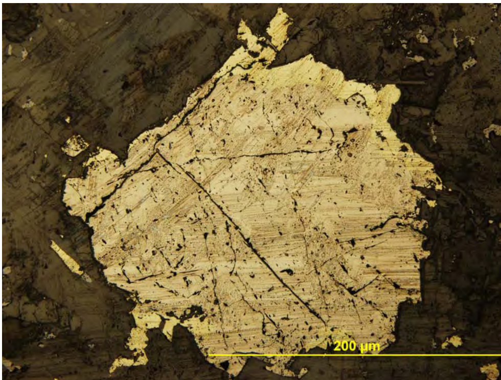
Figure 3.33: Contact mineralization of melanogabbro with basement iron formation is shown in sample ED-10, where up to 2.5 mm blebby immiscible pyrrhotite-chalcopyrite sulphides occur between cumulate crystals.
