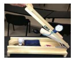
Figure 2. CTCAT device. The device in the open position, with the blue inflation pad, the white hand rest ball, and the black pressure ball.
