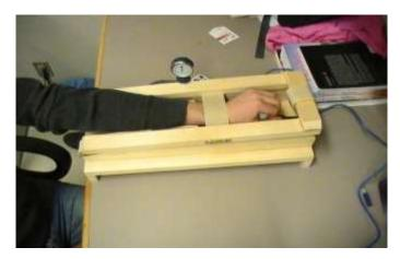
Figure 3. CTCAT testing position. The carpal tunnel space is placed on top of the black pressure ball with the retainer strap on the back of the wrist. The hand rests on the white ball to maintain wrist angle during testing.
