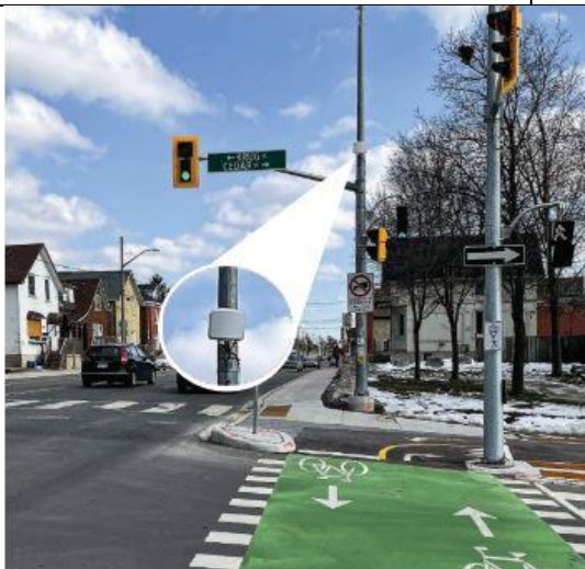
Figure 4.15: A typical implementation of the Wavetronix Bicycle Detection and FORTRAN Wavetronix Bicycle Detection (Source: FORTRAN, 2024).
