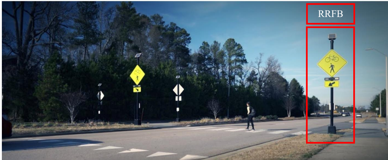
Figure 4.6: Rectangular Rapid Flashing Beacon (RRFB). (Source: Carmanah, 2024).
