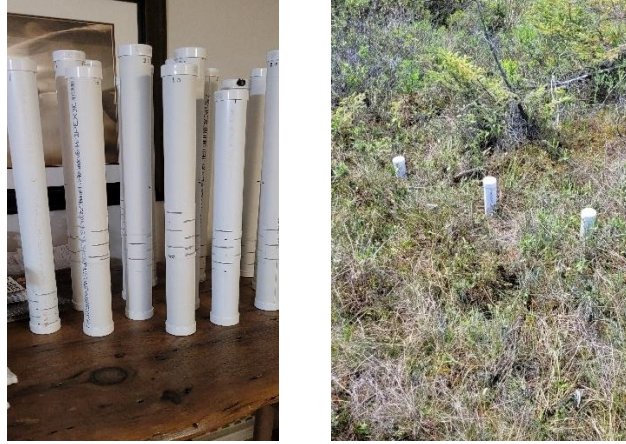
Figure 3.1 A In situ pore water sampling device, B. Example of Piezometer placement in the sampling area
