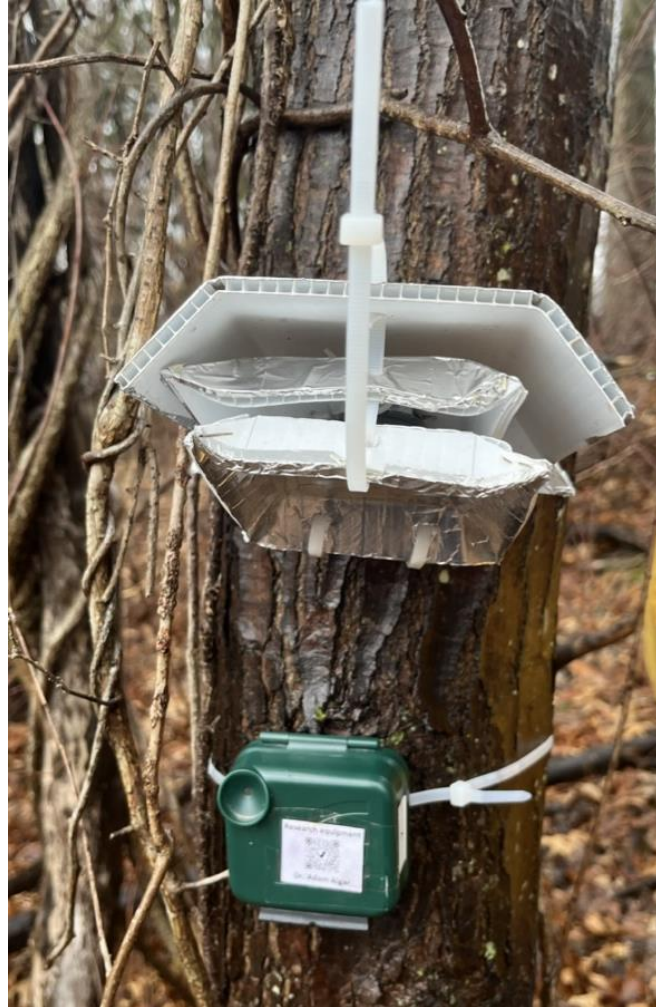
Figure 2.5. Set up for passive acoustic monitoring device (audiomoth) and temperature logger (Hobo MX2201) with radiation shield (Holden et al. 2013).
