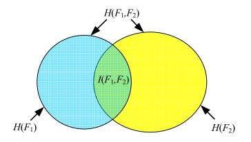
**Figure 4.3.** Illustration of the relationship between entropy  $H(F_1)$  (left circle),  $H(F_2)$  (right circle); mutual information  $I(F_1, F_2)$  (intersection area); and joint entropy  $H(F_1, F_2)$ .
