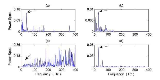
**Figure 5.2.** Comparison of processing results of CWRU dataset of monitoring healthy bearing with a scale of the power spectrum using the technique of: (a) SHHT; (b) WT; (c) HHT; (d) NHHT. (Arrow indicates the characteristic frequency)
