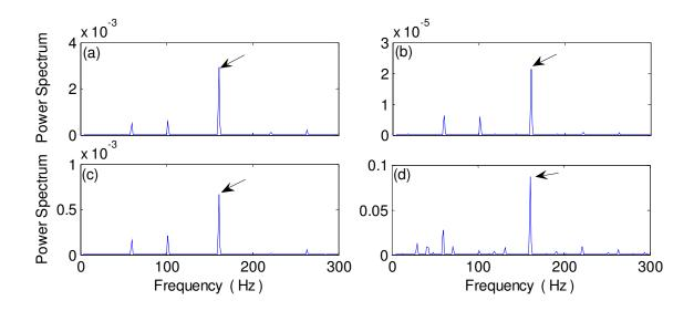
**Figure 5.8.** Comparison of processing results of CWRU dataset for bearing with inner race fault detection using the techniques of: (a) MED-eHHT; (b) eHHT; (c) MED-HHT; (d) MED-WT. (Arrows point to the defect frequency and its harmonics).
