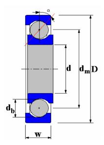
Figure 2.2. Geometry of ball bearing [33].
