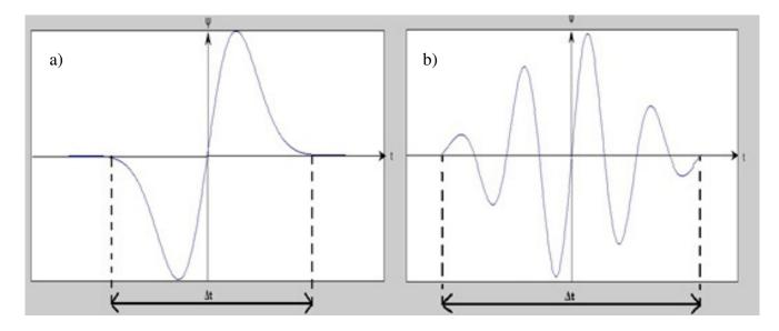
Figure 2.3. Wavelet transformation (WT): compared basis functions with compression factor [34].
