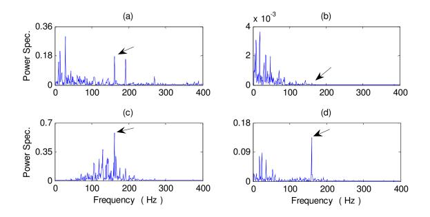
**Figure 5.5.** Comparison of processing results of CWRU dataset for bearing with rolling element (ball) fault detection with a scale of the power spectrum using the techniques of: (a) SHHT; (b) WT; (c) HHT; (d) NHHT. (Arrow indicates the characteristic frequency)
