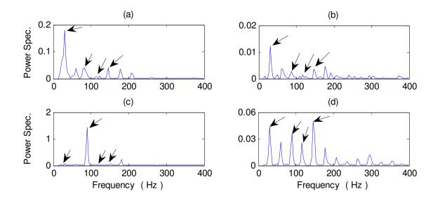
**Figure 5.10.** Comparison of processing results for bearing with combination of all faults detection with a scale of the power spectrum using the techniques of: (a) SHHT; (b) WT; (c) HHT; (d) NHHT. (Arrow indicates the characteristic frequency)
