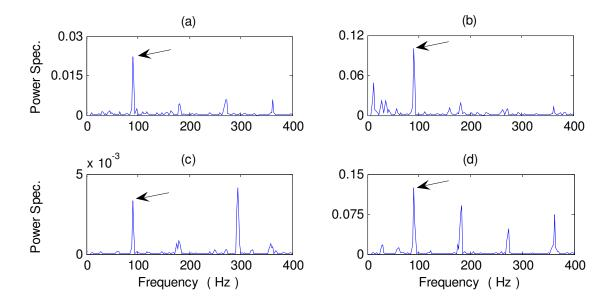
**Figure 3.7.** Comparison of processing results for a bearing with outer race fault detection with a scale of the power spectrum using the techniques of: (a) SHHT; (b) WT; (c) HHT; and (d) NHHT. (Arrow indicates the characteristic frequency)
