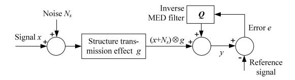
Figure 2.5. Inverse filtering process of MED.
