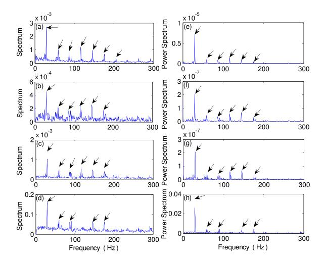
**Figure 4. 5.** Comparison of processing results for a healthy bearing using the related techniques: (a,e) MED-eHHT; (b,f) eHHT; (c,g) MED-HHT; (d,h) MED-WT. The results in the right column are scaled using spectral amplitude, and the results in the left column are with a scale of power spectrum. (Arrows point to the shaft speed and its harmonics)
