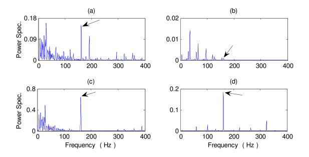
**Figure 5.4.** Comparison of processing results of CWRU dataset for bearing with inner race fault detection with a scale of the power spectrum using the techniques of: (a) SHHT; (b) WT; (c) HHT; (d) NHHT. (Arrow indicates the characteristic frequency)
