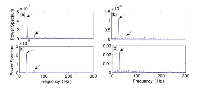
**Figure 5.6.** Comparison of processing results of CWRU dataset of monitoring healthy bearing using the technique of: (a) MED-eHHT; (b); eHHT; (c) MED-HHT; (d) MED-WT. (Arrows point to the shaft speed and its harmonics)
