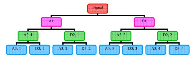
Figure 2.4. Envelope determination using WPT method.
