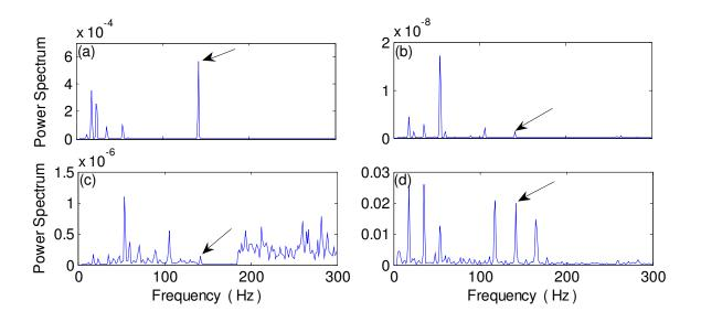
**Figure 4.8.** Comparison of processing results for a bearing with rolling element (ball) fault detection using the techniques of: (a) MED-eHHT; (b) eHHT; (c) MED-HHT; (d) WT. (Arrow points to the defect frequency)
