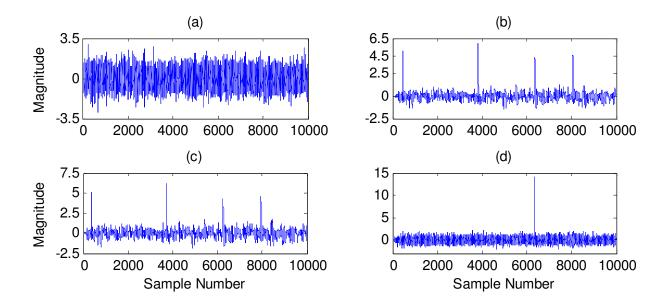
**Figure 4.1.** Response comparison of a test signal using MED filters with different lengths: (a) simulated input signal; (b) MED response with filter length of 100; (c) MED response with filter length of 300; (d) MED response with filter length of 500.
