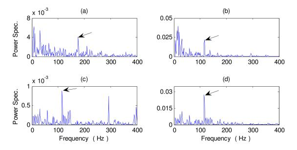
**Figure 3.9.** Comparison of processing results for a bearing with rolling element (ball) fault detection with a scale of the power spectrum using the techniques of: (a) SHHT; (b) WT; (c) HHT; and (d) NHHT. (Arrow indicates the characteristic frequency)
