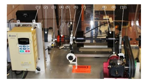
**Figure 3.2.** Verification tests experimental setup: (1) speed control; (2) motor; (3) optical sensor; (4) flexible coupling; (5) ICP accelerometer; (6) bearing housing; (7) test bearing; (8) load disc; (9) magnetic load system; (10) bevel gearbox.
