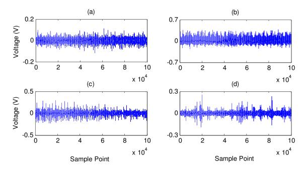
**Figure 3.5.** Part of collected vibration signals for bearings with different health condition: (a) a healthy bearing; (b) a bearing with outer race defect; (c) a bearing with inner race defect; (d) a bearing with rolling element defect.
