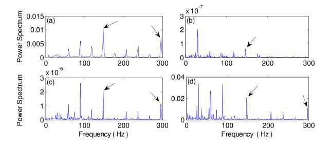
**Figure 4.7.** Comparison of processing results for a bearing with inner race fault detection using the techniques of: (a) MED-eHHT; (b) eHHT; (c) MED-HHT; (d) MED-WT. (Arrows point to the defect frequency and its harmonics)
