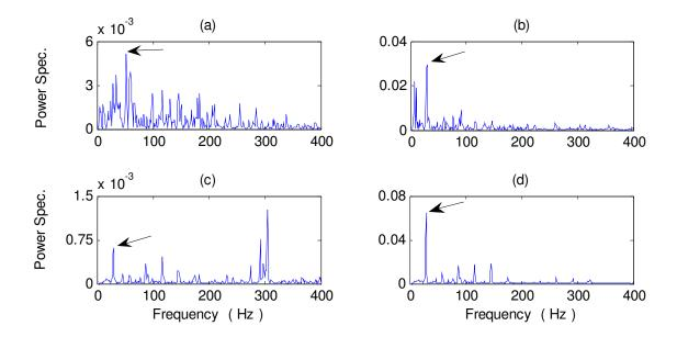
**Figure 3.6.** Comparison of processing results for a healthy bearing using the related techniques with a scale of the power spectrum: (a) SHHT; (b) WT; (c) HHT; and (d) NHHT. (Arrow indicates the characteristic frequency)
