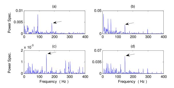
**Figure 3.8.** Comparison of processing results for a bearing with inner race fault detection with a scale of the power spectrum using the techniques of: (a) SHHT; (b) WT; (c) HHT; and (d) NHHT. (Arrow indicates the characteristic frequency)
