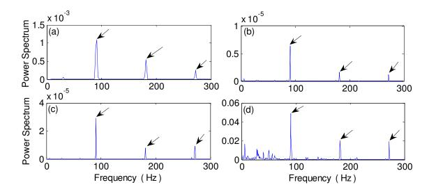
**Figure 4.6.** Comparison of processing results for a bearing with outer race fault detection using the techniques of: (a) MED-eHHT; (b) eHHT; (c) MED-HHT; (d) MED-WT. (Arrows point to the defect frequency and its harmonics)
