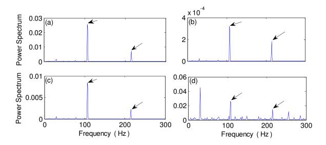
**Figure 5.7.** Comparison of processing results of CWRU dataset for bearing with outer race fault detection using the techniques of: (a) MED-eHHT; (b) eHHT; (c) MED-HHT; (d) MED-WT. (Arrows point to the defect frequency and its harmonics)
