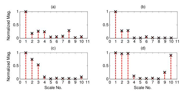
**Figure 3.4.** Demonstration of normalized DP indicator values versus IMF scale numbers corresponding to different bearing health conditions: (a) healthy bearing; (b) bearing with outer race defect; (c) bearing with inner race defect; (d) bearing with rolling element defect.
