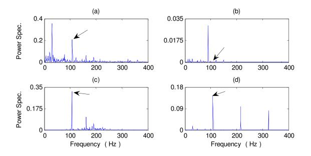
**Figure 5.3.** Comparison of processing results of CWRU dataset for bearing with outer race fault detection with a scale of the power spectrum using the techniques of: (a) SHHT; (b) WT; (c) HHT; (d) NHHT. (Arrow indicates the characteristic frequency)
