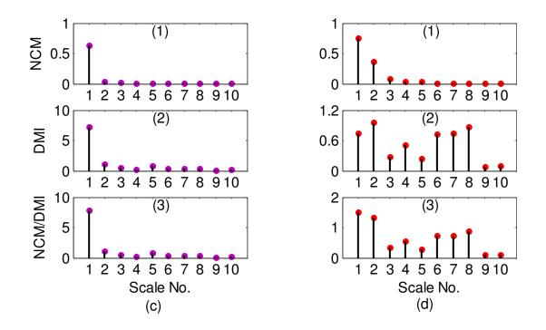
**Figure 4.4.** Demonstration of NCM/DMI indicator values versus IMF scale numbers corresponding to different bearing health conditions: (a1,a2,a3)-healthy bearing; (b1,b2,b3)-bearing with outer race defect; (c1,c2,c3)-bearing with inner race defect; (d1,d2,d3)-bearing with rolling element defect.
