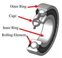
Figure 2.1. Ball bearing structure [32].
