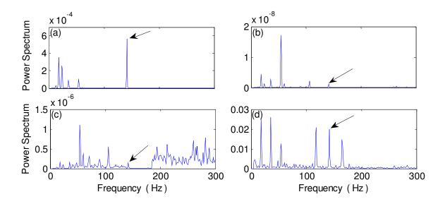
**Figure 5.9.** Comparison of processing results of CWRU dataset for bearing with rolling element (ball) fault detection using the techniques of: (a) MED-eHHT; (b) eHHT; (c) MED-HHT; (d) MED-WT. (Arrow points to the defect frequency)
