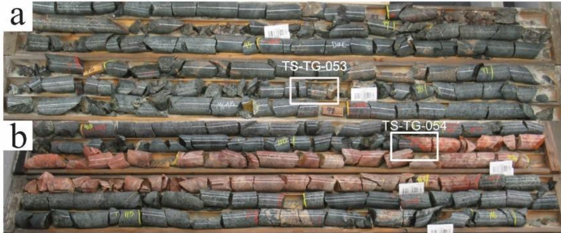
Figure 4.9. Pictures of wet drill core from hole RR004-003. a) 92.06-99.61 m, showing the contact sampled for TS-TG-053 of melagabbro and a pegmatitic felsic veinlet. b) 107.85-116.04 m, showing the contact sampled for TS-TG-054 of melagabbro and felsic dike.
