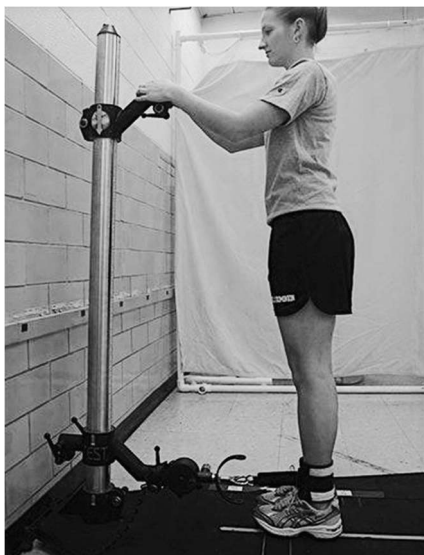
Figure 9. Standing Testing Procedure . The Evaluator™ HHD used in standing testing (Kollock et al., 2010).
