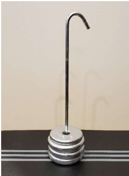
Figure 10. Metal bar which will be used for Part One of testing, including weight plates.
