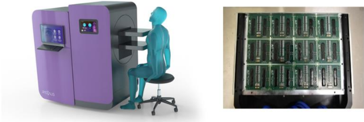
Figure 3.2 - Left: Clinical prototype of PEM camera with two planar detector heads; Right: 3×4 array of sensor modules inside a detector head (bottom).
