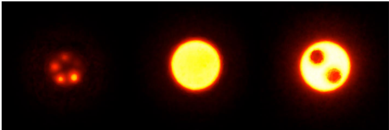
Figure 4.10 - NEMA NU-4 IQ phantom reconstructed using the latest GPU-based reconstruction. Slices displaying the hot rods for recovery coefficient (left), uniform region (center) and air and water reservoirs (right)
