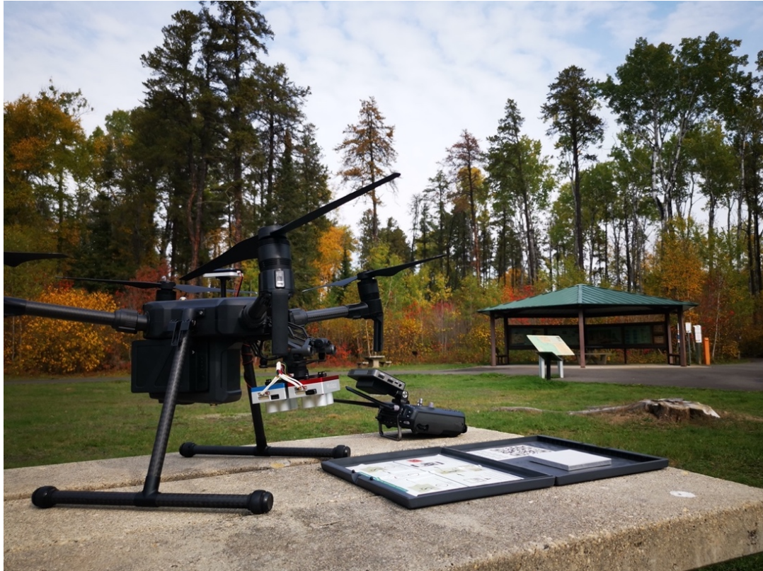
Figure 2. DJI Matrice 200 equipped with the MicaSense dual sensor, accompanied by the CRP 2. The stand being studied is visible in the background, displaying the stand complexity and species mixtures.
