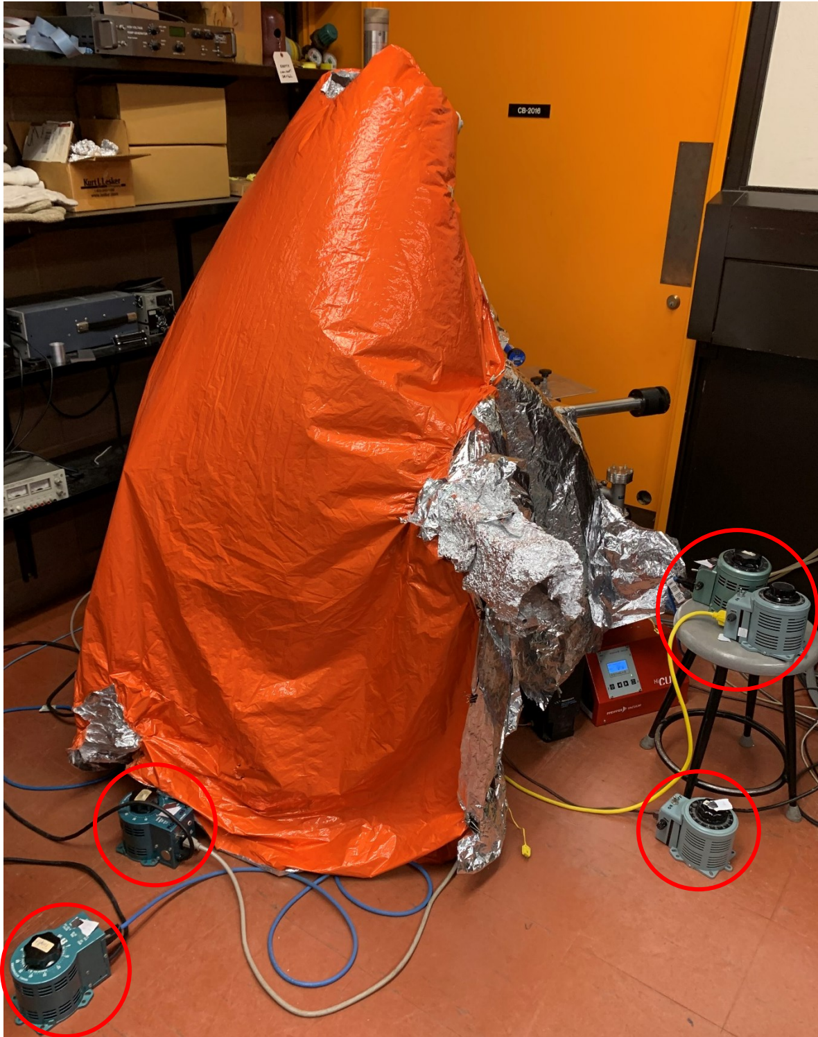
Fig. 4.4: Our UHV chamber during the baking process. Variable AC power supplies are circled in red. Temperatures are monitored with thermocouples.
