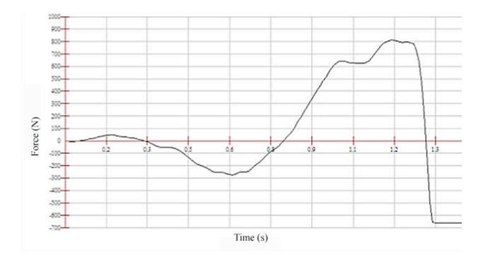
Figure 7: Ground reaction force vs. time during countermovement vertical jump
