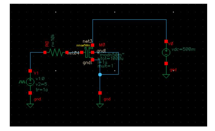
Figure 8.1: Circuit setup to find the gate capacitance
