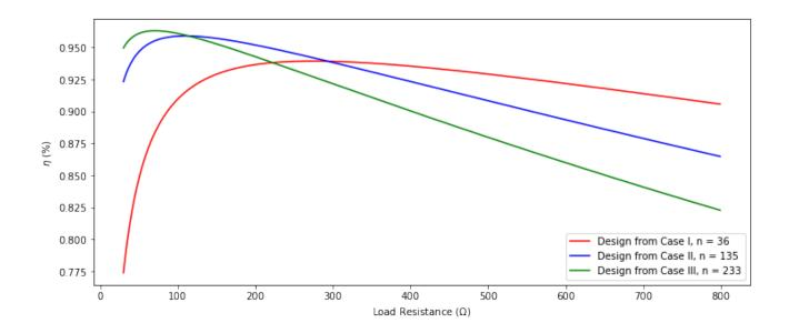
Figure 4.24: Power efficiency vs load resistance
