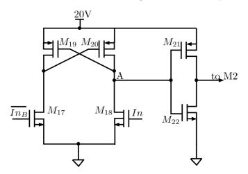
Figure 4.18: 20V Level Shifter design
