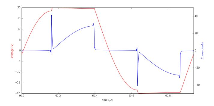
Figure 6.2: Output Voltage and Current of transducer 2
