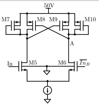
Figure 4.12: Schematic of a conventional level shifter
