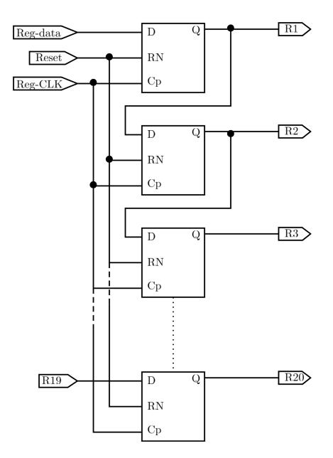
Figure 4.4: Schematic of the 20-bits Register
