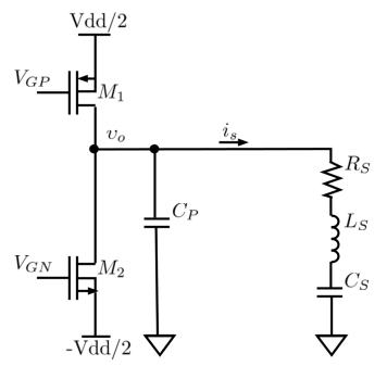
Figure 2.16: Class DE simplified circuit
