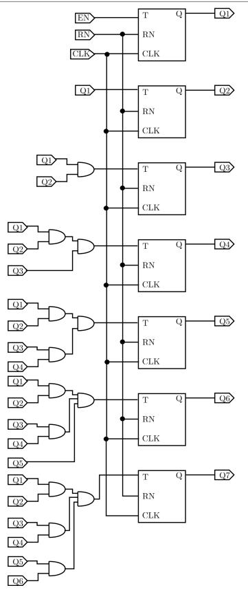
Figure 4.3: Schematic of the 7-bits counter
