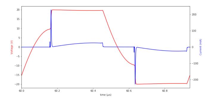
Figure 6.4: Output Voltage and Current of transducer 4
