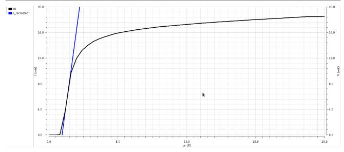
Figure 7.5: measure  $I_D$  (black) and recreated  $I_D$  (blue) with only K parameter for NMOS50M
