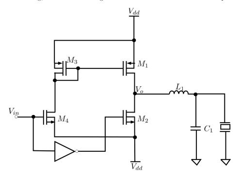
Figure 2.11: Schematic of LIPUS amplifier proposed in [22]
