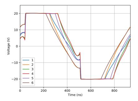
Figure 3.7: Sim 3 Output voltages
