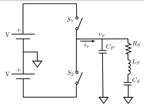
Figure 3.1: Simplified class DE circuit
