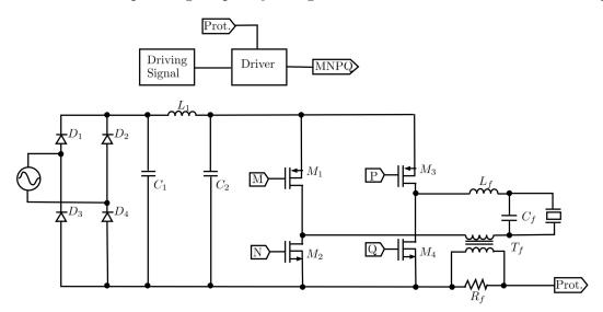
Figure 2.8: Schematic of class D Amplifier proposed by Agbossou [15]
