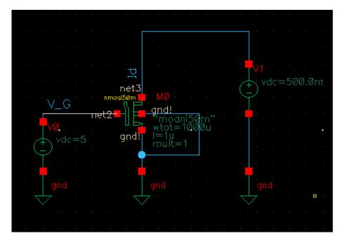
Figure 7.4: Circuit setup to extract parameters for NMOS50M
