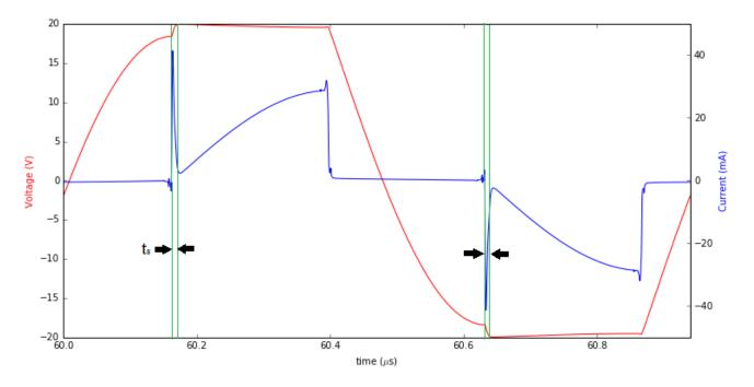
Figure 4.28: Extracting switching loss from simulation, red line is  $v_o$ , and blue line is  $i_s$ The simulation results are very close to the calculations as shown in Table 4.3.
