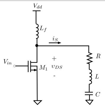
Figure 2.13: Schematic of class E amplifier [14]
