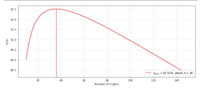
Figure 4.20: Power efficiency vs number of fingers for transducer array used in section 3.3
