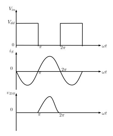
Figure 2.14: Waveforms of class E amplifier [14]
