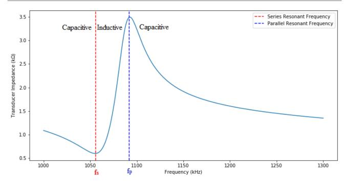
Figure 2.4: Magnitude of the Transducer Impeadance vs Operating Frequency.  $f_s$  is the series resonant frequency, where as  $f_p$  is the parallel resonant frequency [15]
