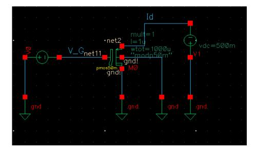
Figure 7.7: Circuit setup to extract parameters for PMOS50M
