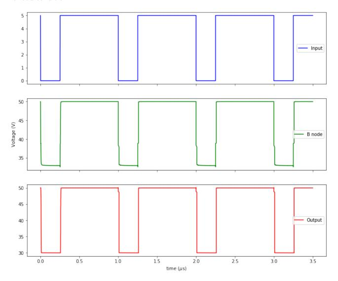
Figure 4.16: Simulated results of the proposed Level Shifter
