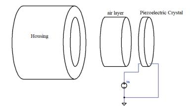
Figure 2.1: Exploded view of a transducer [3]
