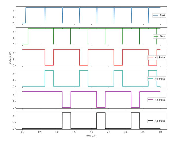
Figure 4.11: Outputs of the Pulse Train Generator
