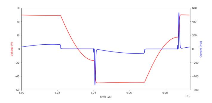
Figure 6.9: Output Voltage and Current of transducer 3
