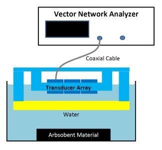
Figure 2.3: Measuring the impedance of the transducers
