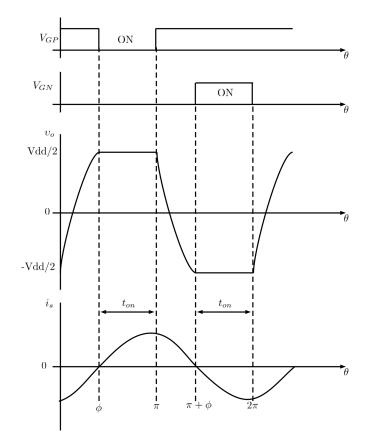
Figure 2.17: Class DE waveform
