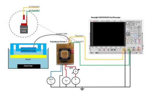
Figure 3.8: Experimental Setup
