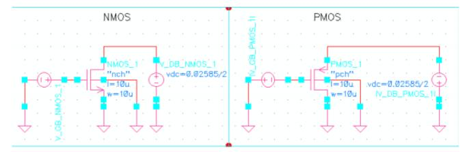
Figure 7.1:  $I_{SQ}$  and  $V_t$  extraction circuit
