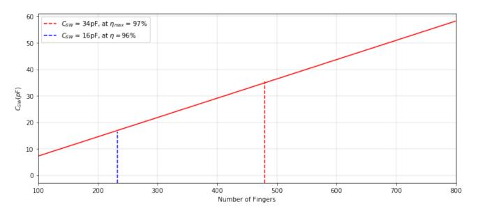
Figure 4.23: Switch capacitance vs number of fingers for transducer array used in section 3.4
