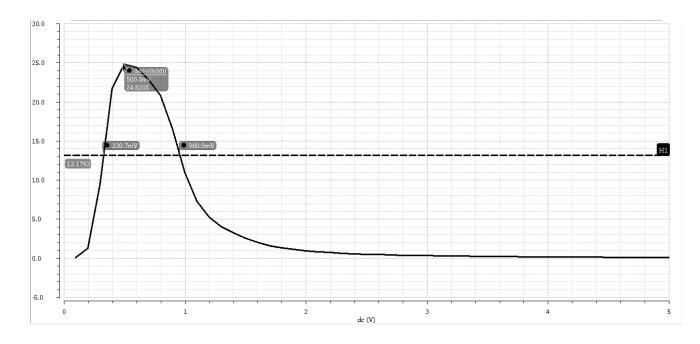
Figure 7.3: Obtaining  $V_t$  for NMOS50M
