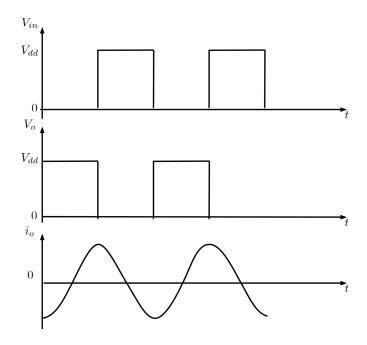
Figure 2.6: Waveforms of class D amplifier [14]
