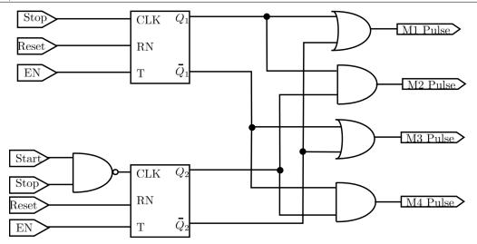
Figure 4.6: Schematic of the Output Block
