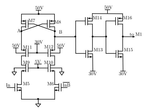
Figure 4.14: Schematic diagram for the 30-50 V level shifter
