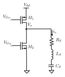
Figure 2.5: Schematic of class D amplifier[14]
