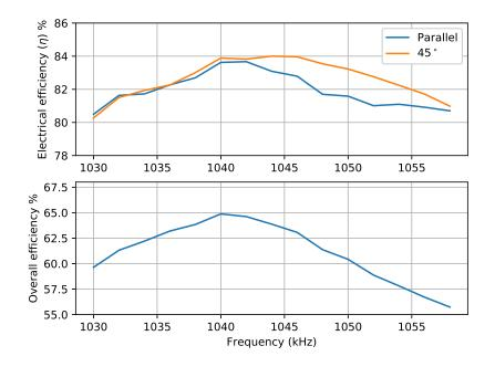
Figure 3.13: Array electrical efficiency  $(\eta)$  and overall combined electrical-acoustic efficiency vs. frequency.
