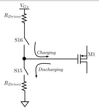
Figure 4.15: Simplified Gate Driving circuit
