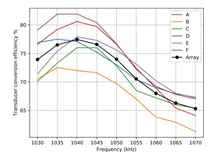
Figure 3.11: Transducer conversion efficiency as a function of frequency.
