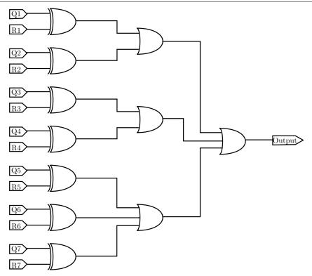
Figure 4.5: Schematic of the 7-bits Comparator
