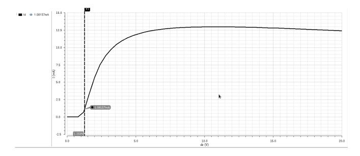
Figure 7.2:  $I_D vsV_{GB}$  for NMOS50M
