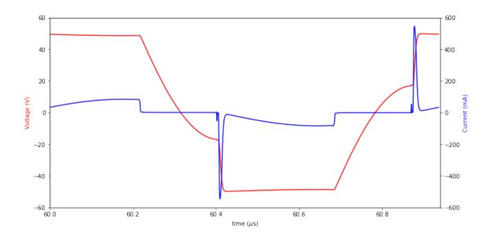
Figure 6.11: Output Voltage and Current of transducer 5
