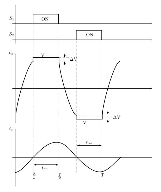
Figure 3.2: Class DE output waveform outside optimum condition
