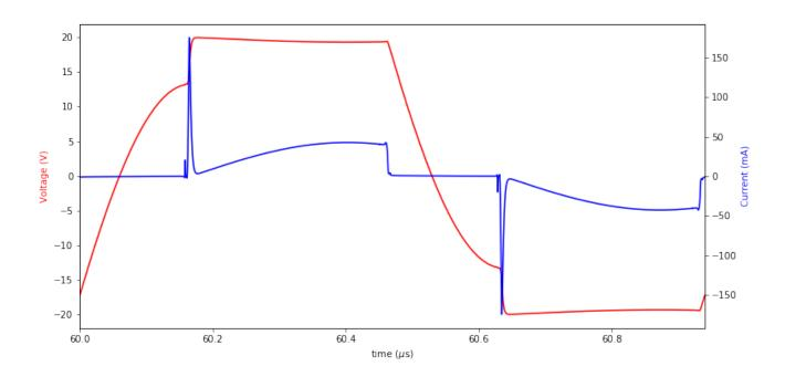
Figure 6.6: Output Voltage and Current of transducer 6
