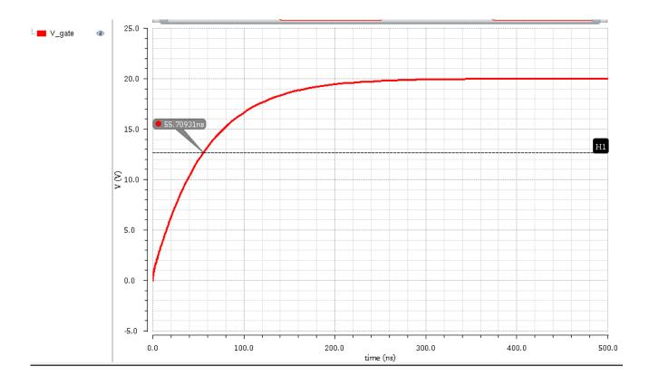
Figure 8.2: Gate capacitance charging curve
