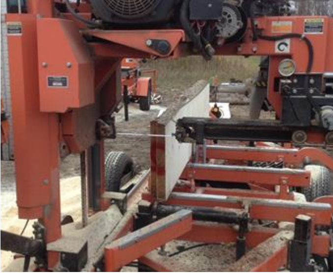
Figure 8. Removal of bark from 1” boards using the Wood-Mizer LT40H.
