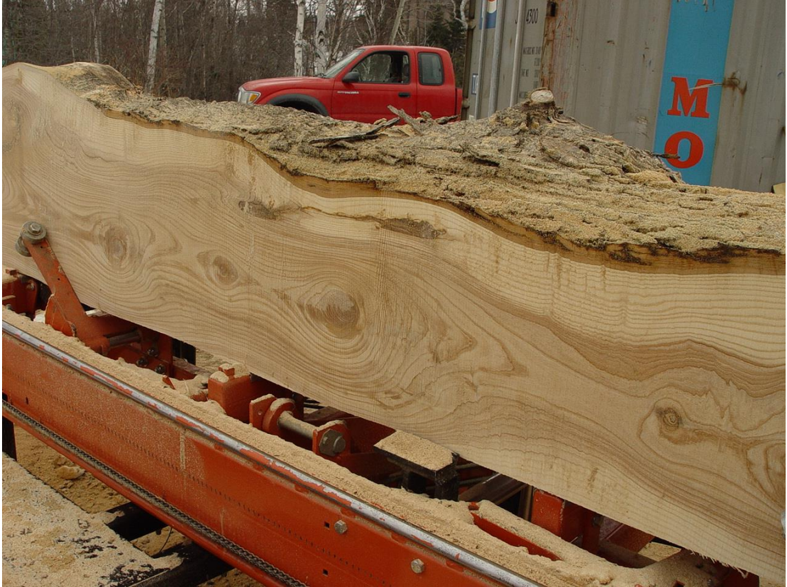
Figure 3. A partially milled green ash log. Heartwood is a variable light-brown colour in contrast with the light and pale sapwood on the margins of the log.
