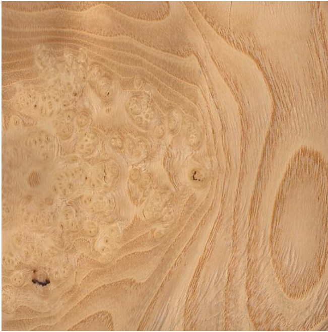
Figure 4. Burlwood surrounded by heartwood from an ash tree (The Wood Database 2018a).
