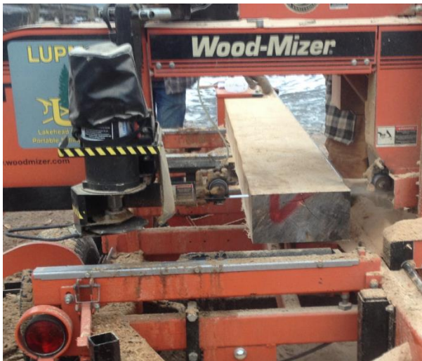
Figure 10. Green ash log milled using the quarter saw (canting) method.
