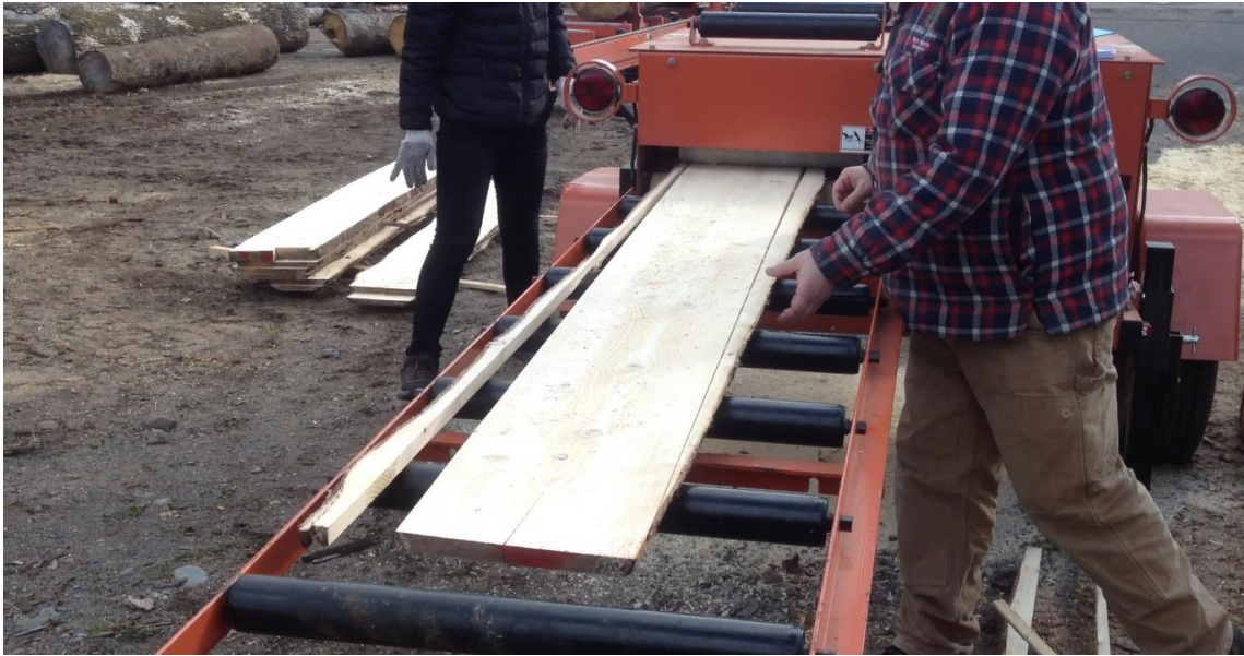
Figure 7. Removal of bark from 1" boards using the Wood-Mizer Twin Blade Edger.
