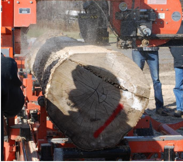
Figure 9. A green ash log being milled using the canting method. This log would need a couple more cuts at 1" thickness to finish one side of the cant.
