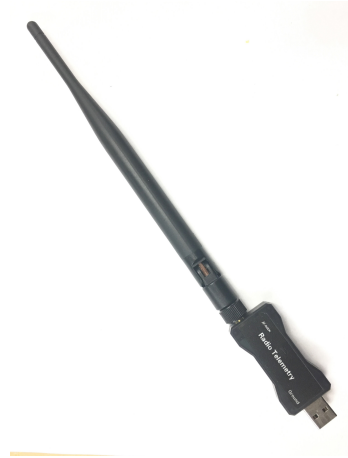
Figure 2.8: 2.4 Ghz Wireless Data Transfer Radio
