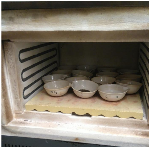
Figure 12. Soil samples inside of the muffle furnace.
