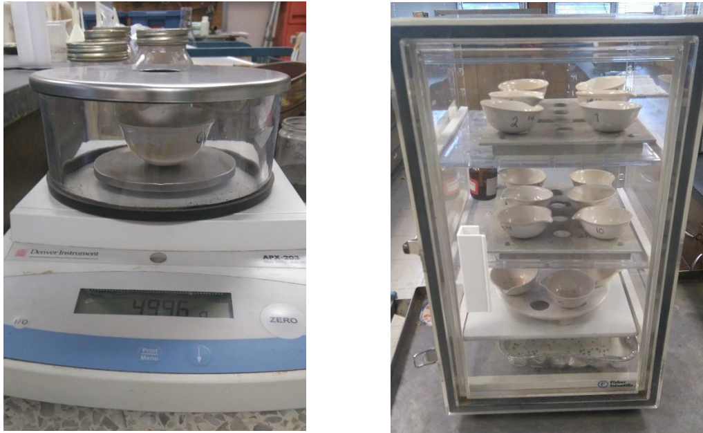
Figure 10. Soil sample being weighed using the APX-203 3-point scale (Left) and porcelain crucibles in the desiccator (Right).
