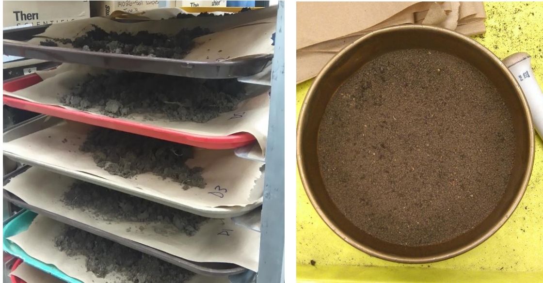
Figure 9. Air drying of soil samples (Left) and fully prepared soil sample (Right).
