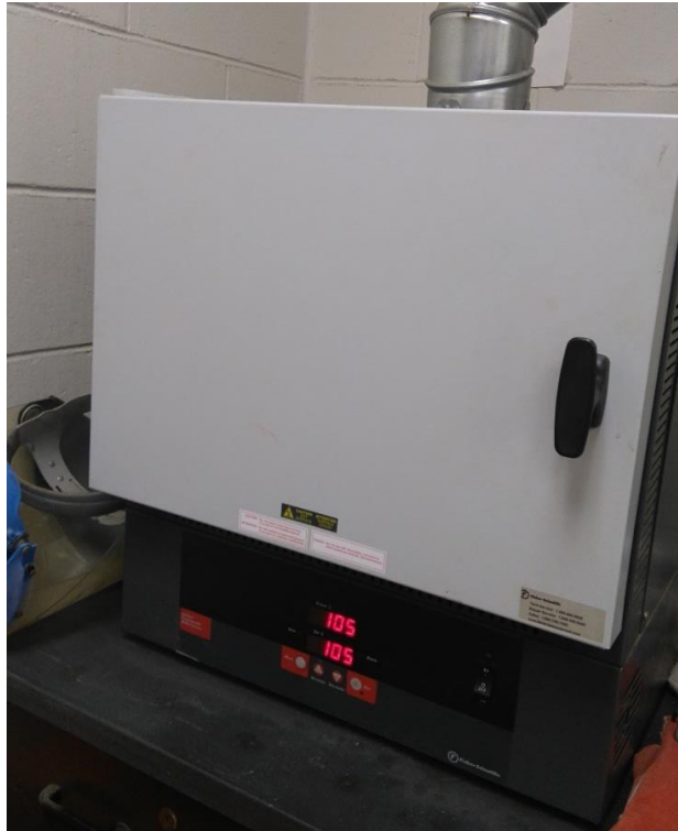
Figure 11. Fisher Scientific Isotemperature Programmable Muffle Furnace.
