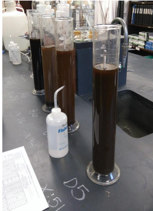
Figure 19. Soil samples in the sedimentation cylinders.
