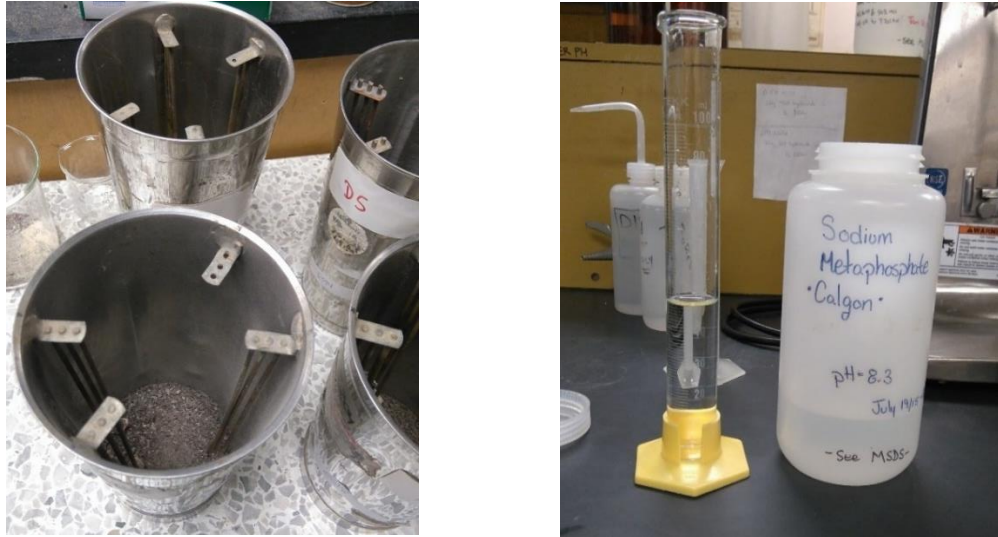
Figure 17. Soil samples in the dispersion cups (Left) and Calgon (Sodium metaphosphate).
