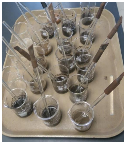
Figure 14. Soil samples mixed with \text{CaCl}_2 solution.
