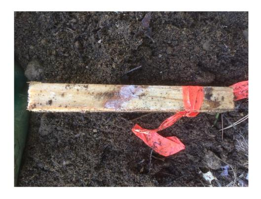
**Figure 21.** Picture of woodblock from DRI on May 13, 2018, white hyphae from *H. fasciculare* visible.
