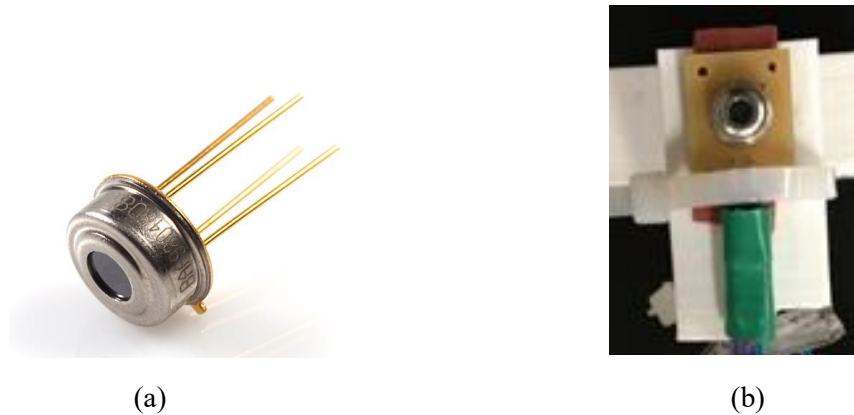
Figure 4.3. Diagrams of (a) IR temperature sensor, (b) Temperature sensor with pinboard (retrieved from [38]).
