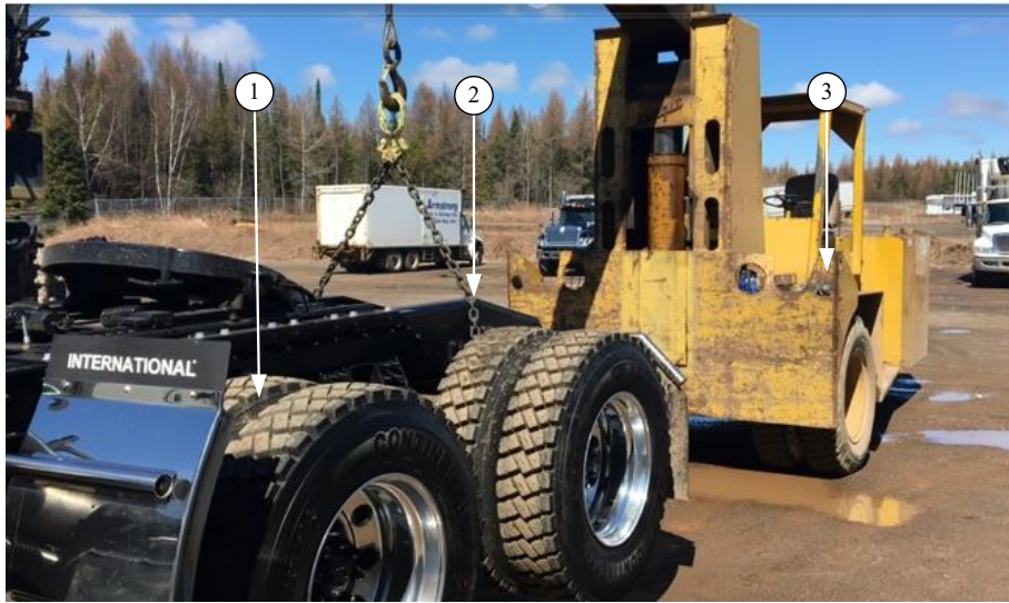
Figure A.2. Speed sensor testing investigation performed in Maxim Truck & Trailer company: (1)Transportation truck, (2) Rear axle towed, (3) Industrial towing vehicle.
