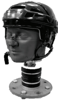
Figure 9. NOCSAE headform fitted with an ice hockey helmet.
