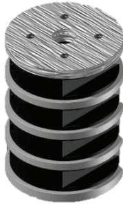
Figure 10. Mechanical neckform. This custom neckform can be attached to a NOCSAE headform and together simulate the dynamic response human experience upon impact.
