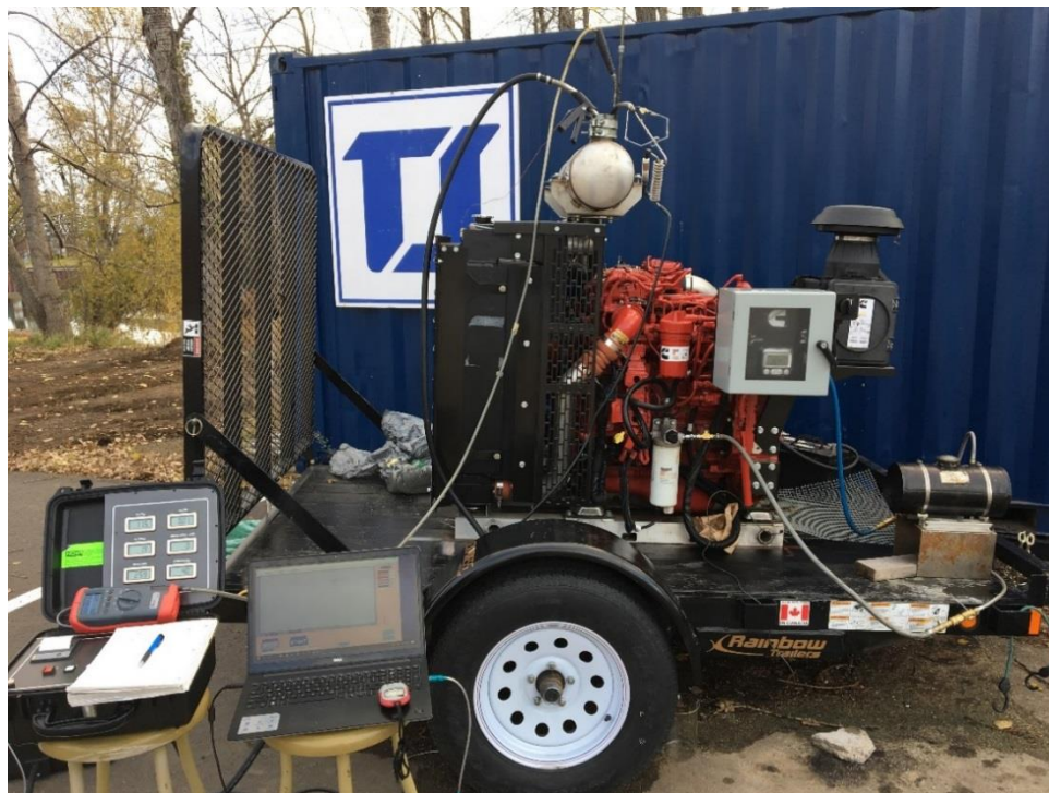
Figure 3.1: Heavy-duty engine test setup
