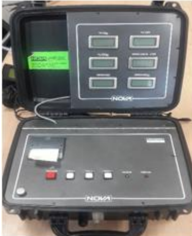
Figure G.5 multi-gas analyzer.
