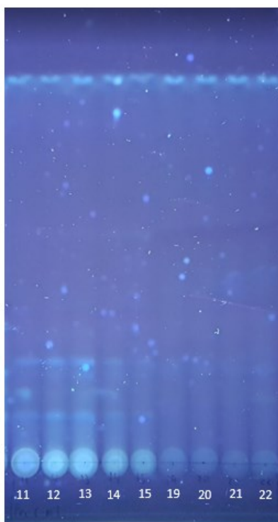
Figure 4-6: TLC of SG60 Fraction #6 Sephadex LH-20 Separated Fractions. Solvent used was 170:30 toluene:acetic acid, plate used was silica gel 60 glass backed TLC plate, plate is illuminated with 365 nm UV light.
