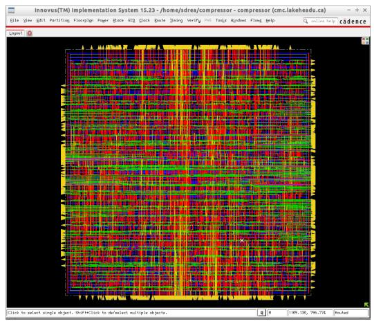
Figure 4.9 – Compressor Routing in Innovus
