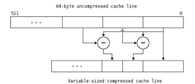
Figure 3.3 – Compressor Design
