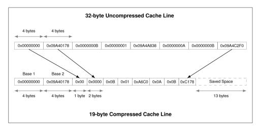
Figure 2.3 – 32-Byte Cache Line Compressed with Base-Delta (2 Bases)
