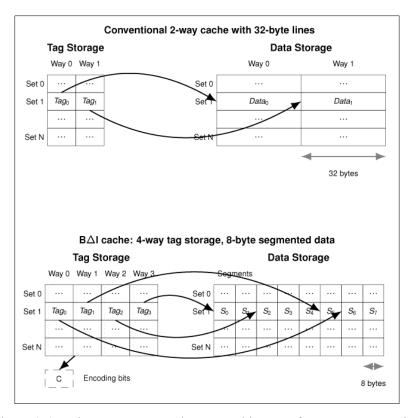
Figure 2.4 – Changes to Tag and Data Architecture for BΔI Compression
