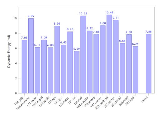
Figure 5.10 – L1 Data Cache Dynamic Energy (Compressed Scheme)
