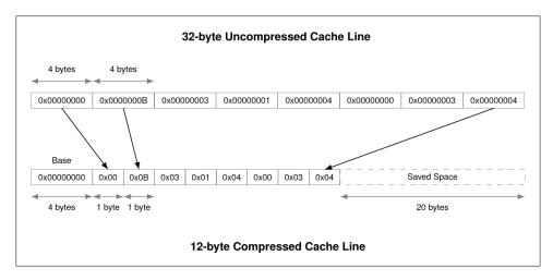
Figure 2.2 – 32-Byte Cache Line Compressed with Base-Delta
