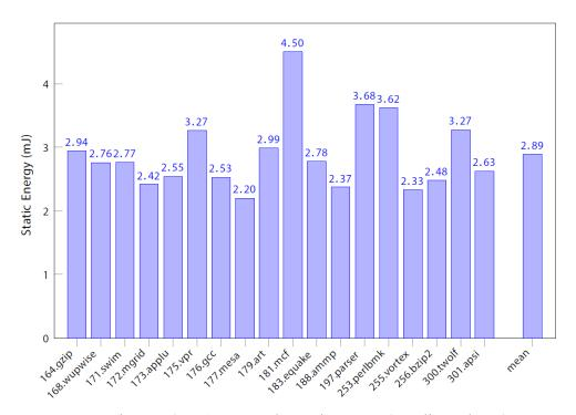
Figure 5.6 – L1 Data Cache Static Energy (Baseline Scheme)
