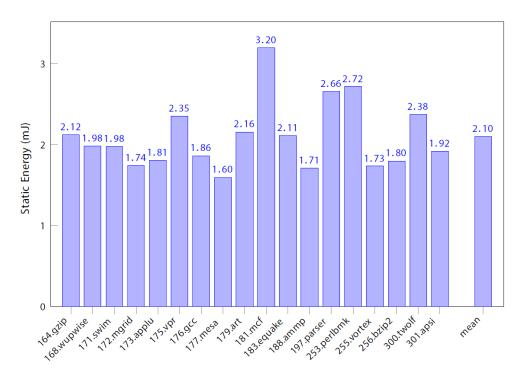
Figure 5.7 – L1 Data Cache Static Energy (Compressed Scheme)
