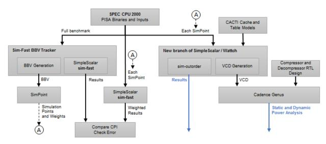
Figure 4.1 – Simulation Flow Diagram
