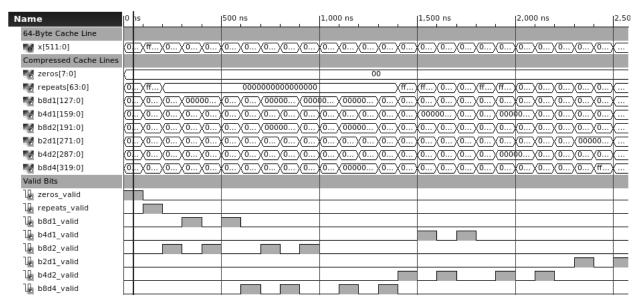
Figure 3.9 – Testbench Waveforms for Compressor in Xilinx ISE
