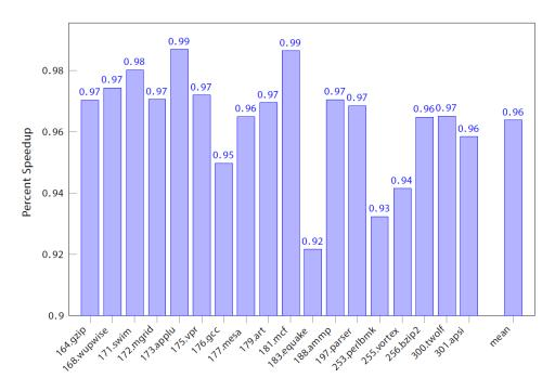
Figure 5.5 – Speedup of Compressed Scheme vs Baseline
