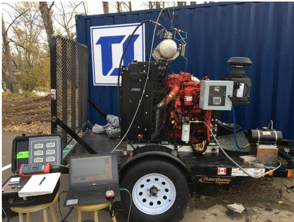
Figure 3.7: Heavy-duty engine test setup
