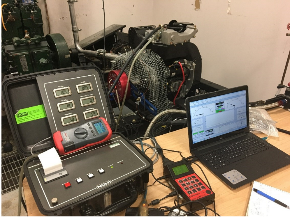
Figure 3.9: Light-duty engine test setup
