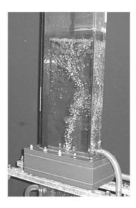
Figure 2.2: The rectangular bubble column reactor of experiment of Pfleger et al. (1999).
