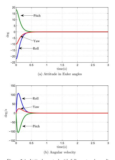
Figure 5.4: Attitude control with fully vector decoupling
