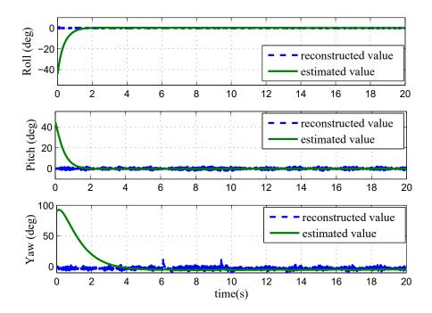
Figure 4.6: Real-time estimation for static attitude
