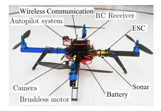
Figure 3.2: Overview of the quadrotor hardwares
