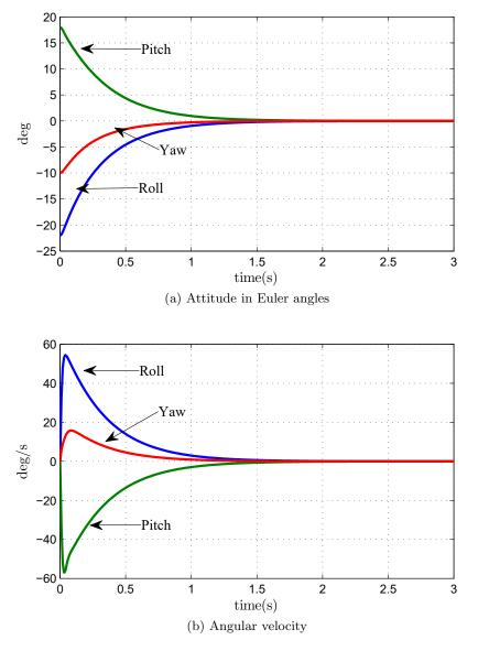
Figure 6.8: Attitude control with standard velocity-free approach
