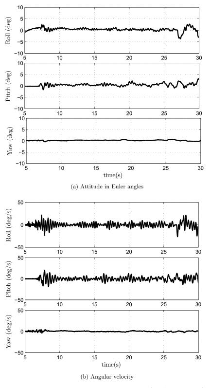
Figure 5.8: Attitude stabilization with controller (5.41) and filter (5.53)
