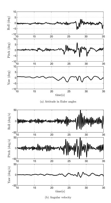
Figure 5.7: Attitude stabilization with controller (5.32) and filter (5.56)
