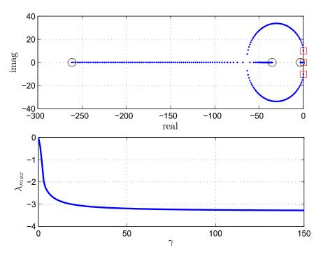
Figure 6.3: Eigenvalues of the yaw dynamics varying with  $\gamma$
