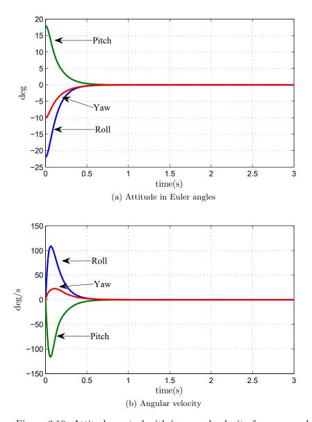
Figure 6.10: Attitude control with improved velocity-free approach
