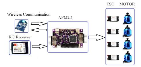
Figure 3.3: Diagram of the quadrotor hardwares
