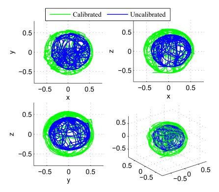
Figure 3.12: Magnetometer calibration results
