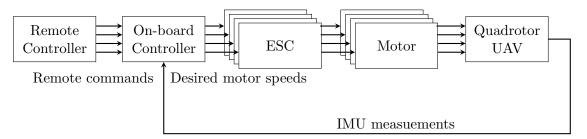
Figure 3.13: Overview of the quadrotor cascaded control loop
