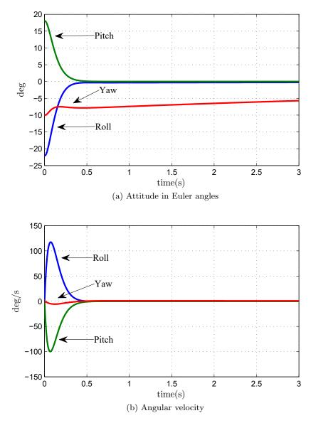
Figure 5.2: Attitude control without vector decoupling
