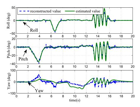
Figure 4.7: Real-time estimation for time-varying attitude
