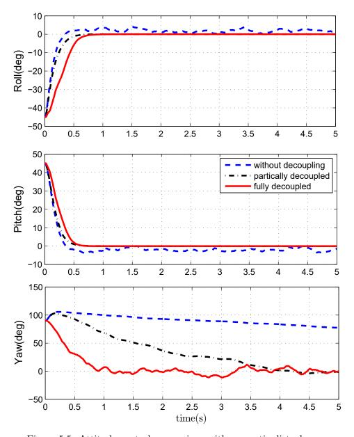
Figure 5.5: Attitude control comparison with magnetic disturbances
