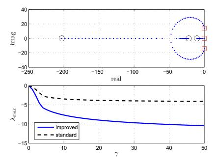
Figure 6.5: Eigenvalues of the pitch dynamics varying with gamma
