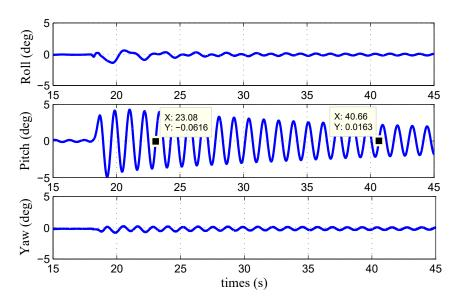
Figure 3.8: Test 1: oscillation around x axis
