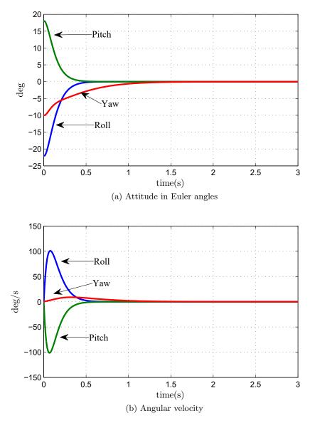
Figure 5.3: Attitude control with partially vector decoupling
