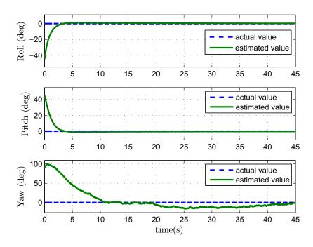
Figure 4.1: Static attitude estimation with gyro-bias
