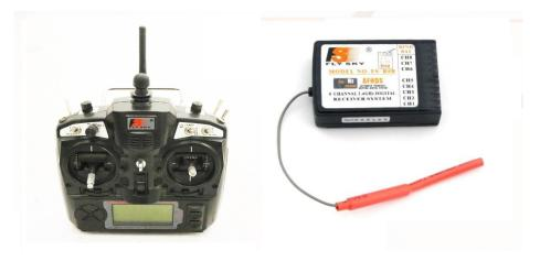
Figure 3.5: Transmitter FS-TH9X (left) and receiver FS-R8B (right)
