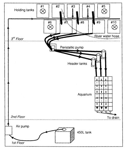
Figure 5 – Diagram of the bioassay setup at AbitibiBowater - Thunder Bay.
