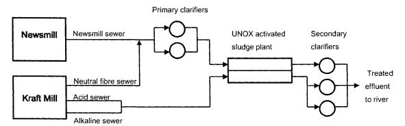
Figure 4 – Effluent treatment process of AbitibiBowater - Thunder Bay (modified from Hardy 2002).
