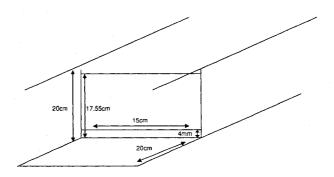
Figure 9 - Dimensions of a compartment within the flow through aquarium. Each compartment housed a breeding pair of fathead minnows and a spawning substrate (modified from Hardy 2002).
