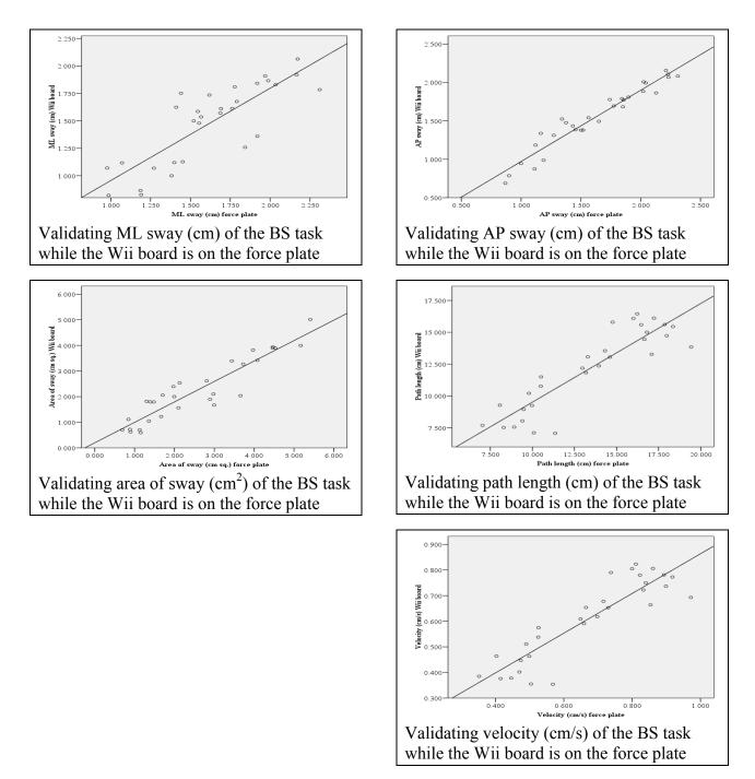
*Figure 8*. Validating COP measures of the balance space (BS) task while the Wii board is on the AMTI force plate.
