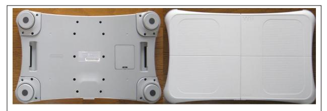
*Figure 21*. Wii board. The board on the left illustrates that the four sensors are in the corners of the board. The board on the right shows the rectangles where the individual should stand while performing simulations. Adapted from "About the Wii console" by Nintendo, 2010. Copyright 2010 by author, Canada.
