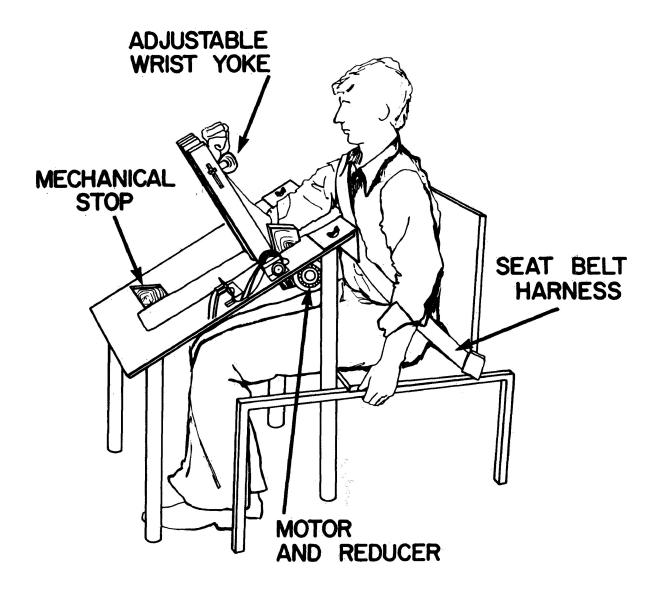
Figure 1. Dynamometer for Testing and Training.
