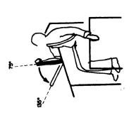
Chest plate adjusted to insure that the joint axis coincides with the instrument axis.
