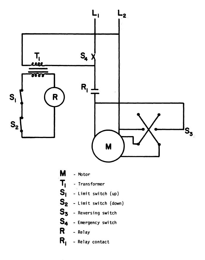
Figure 4. Motor Circuit Diagram.
